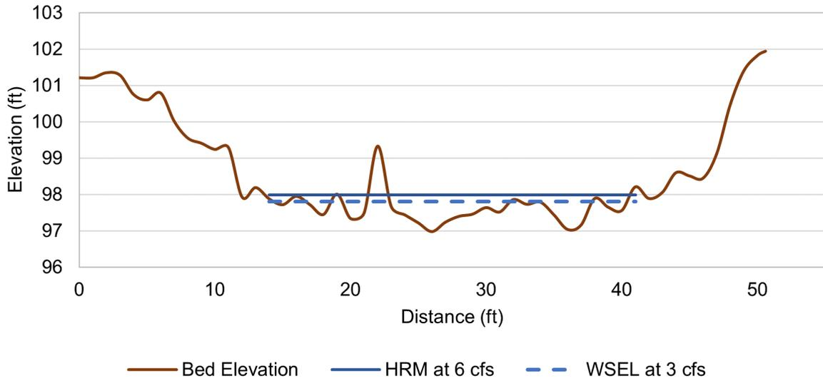
Figure B-13. Mark West Creek 3HRM3 transect cross section with bed elevation, WPM WSEL, and HRM WSEL.
