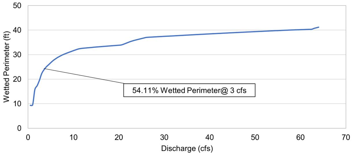
Figure B-14. Mark West Creek 3HRM3 transect wetted perimeter-discharge curve.
