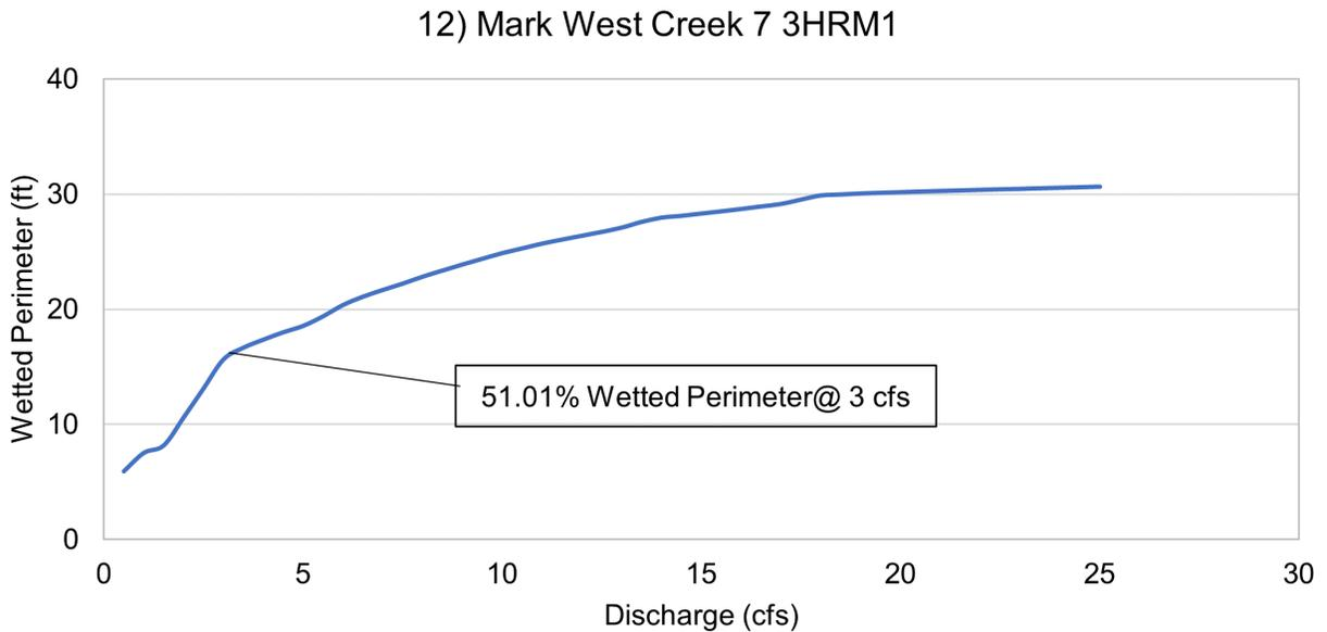
Figure B-12. Mark West Creek 3HRM1 transect wetted perimeter-discharge curve.
