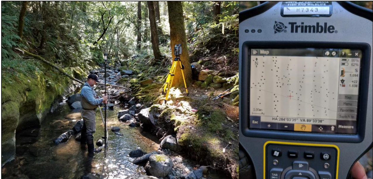
Figure 12. Total station surveying (left) and example of unbalanced survey point density (right). Photo from Mark West Creek Site 3.
