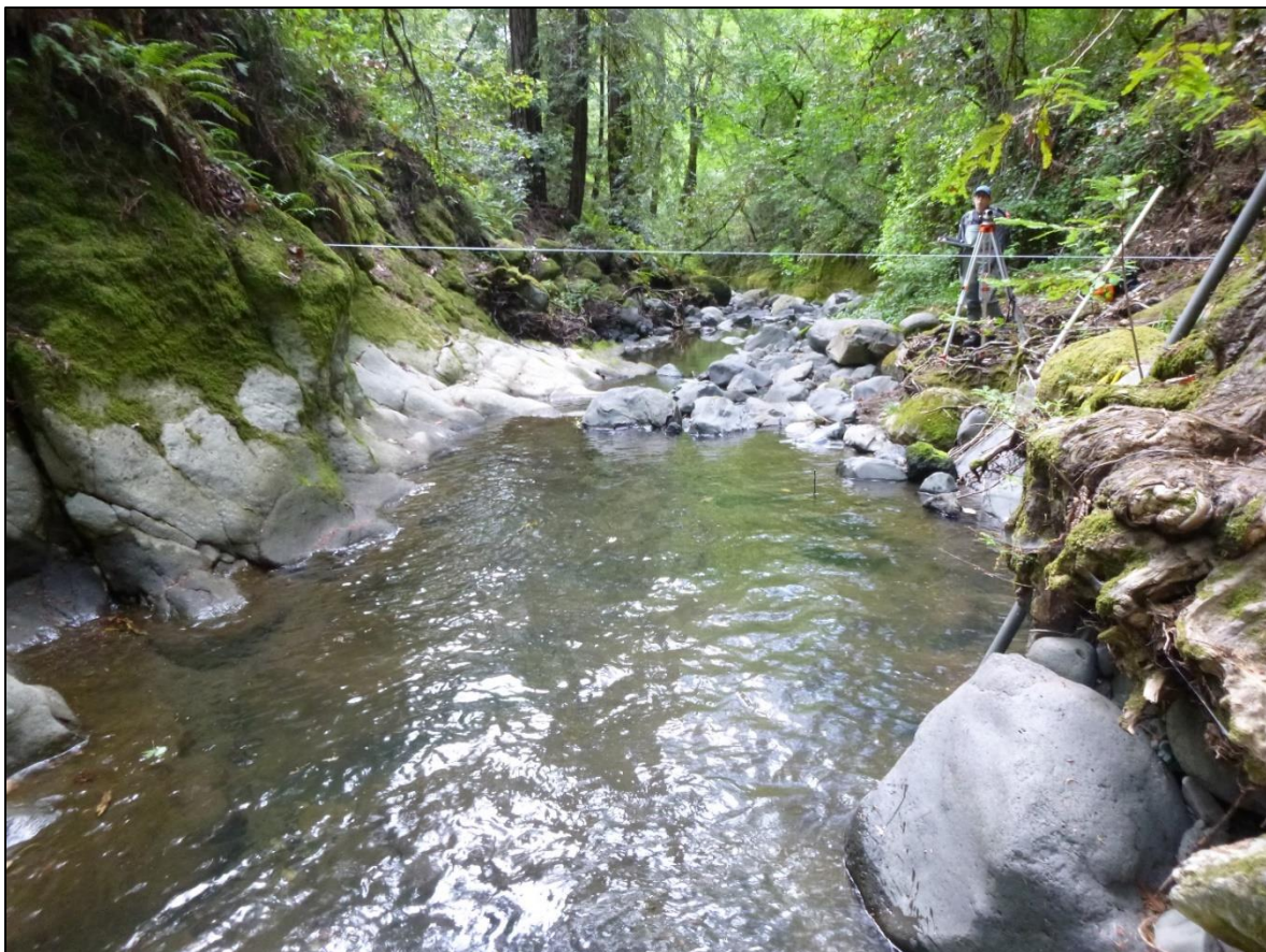
Figure 13. Transect field survey with fiberglass tape and auto level at the downstream boundary (XS-1) of Site 3.
