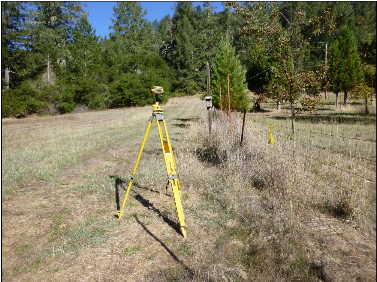
Figure 10. Static survey using RTK-GPS rover in an area near a site with an unobstructed view of the sky.
