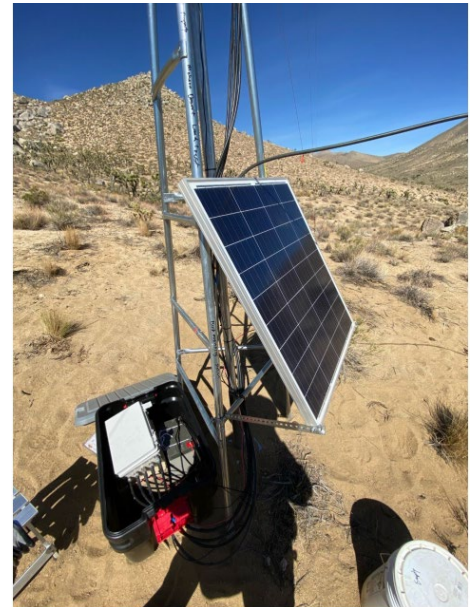
Photo to Right: Motus unit for avian monitoring installed at Frog Spring
