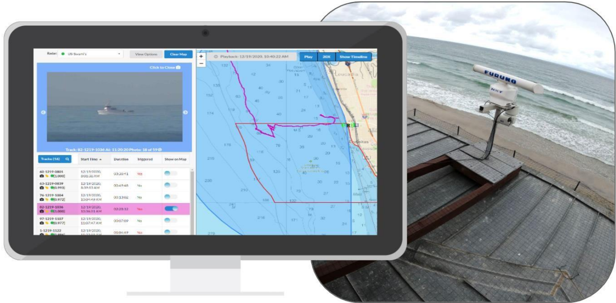
Figure 1. M2 system in Encinitas. This system is deployed at the Moonlight Beach Marine Safety Center and tracks vessels in the vicinity of the Swami's State Marine Conservation Area with both live and historical data accessible from anywhere with the M2 Viewer.
