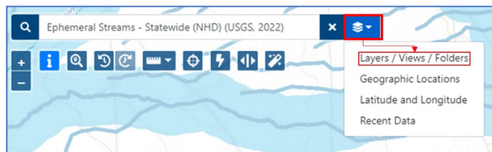
Figure 7. Use the Search Bar to find data layers displaying specific stream types (ephemeral, intermittent, perennial) to enter the stream type you are interested in. Note that you will need to select the dropdown menu and choose the “Layers/Views/Folders” option first. The symbology of the stream-specific layers is shown on the right.
