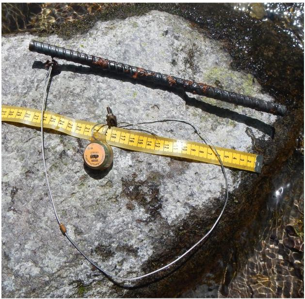
Figure 23. Onset Tidbit water temperature logger setup (without protective cover boot).
