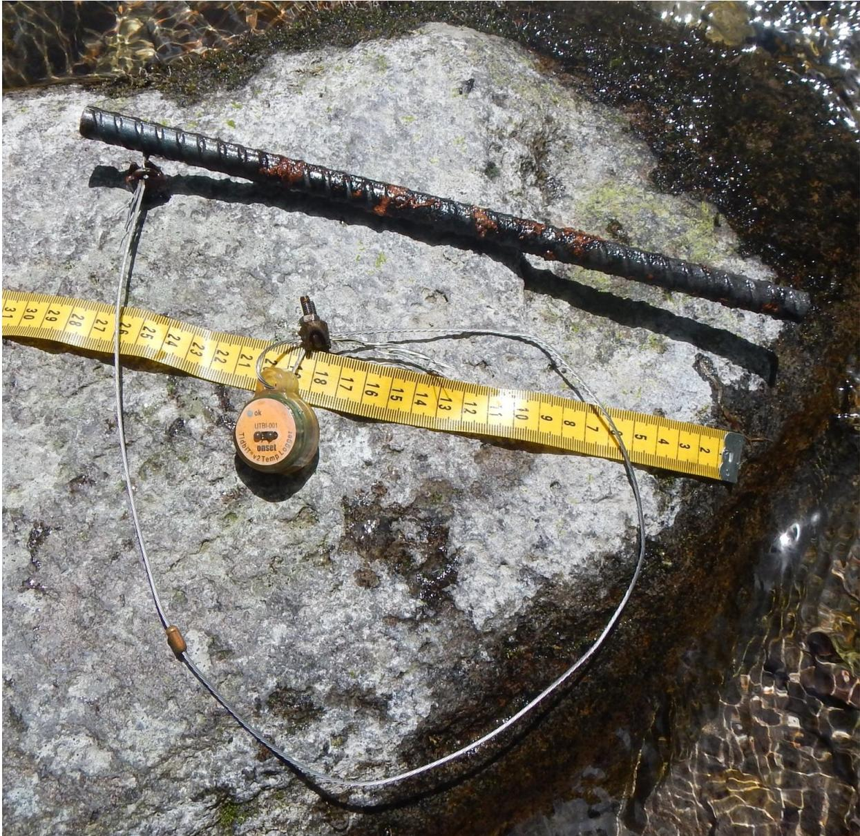
Figure 23. Onset Tidbit water temperature logger setup (without protective cover boot).
