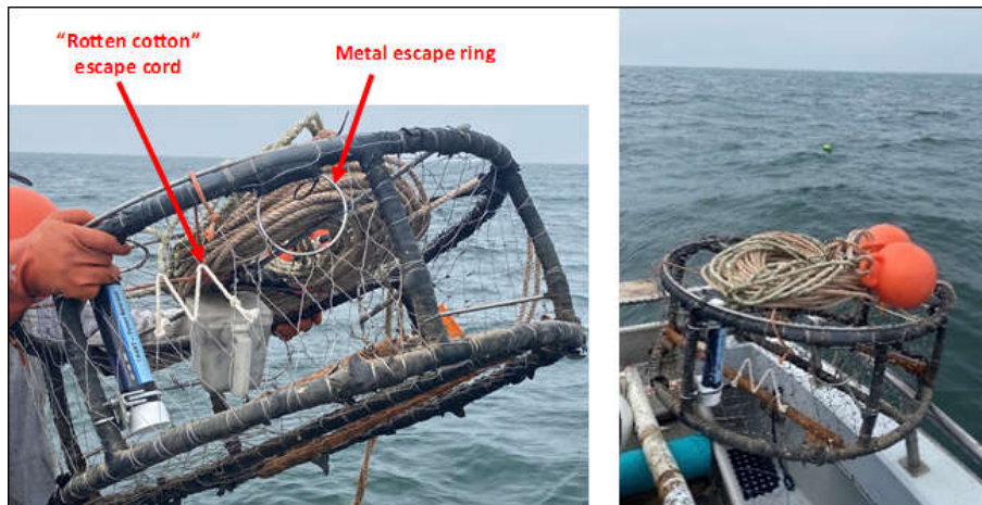
Figure 7. Configuration including degradable “rotten cotton” and steel escape ring installed on the side of the trap.
