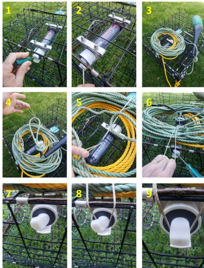
Figure 6. Typical rigging sequence for the TR4RT line handling system.
