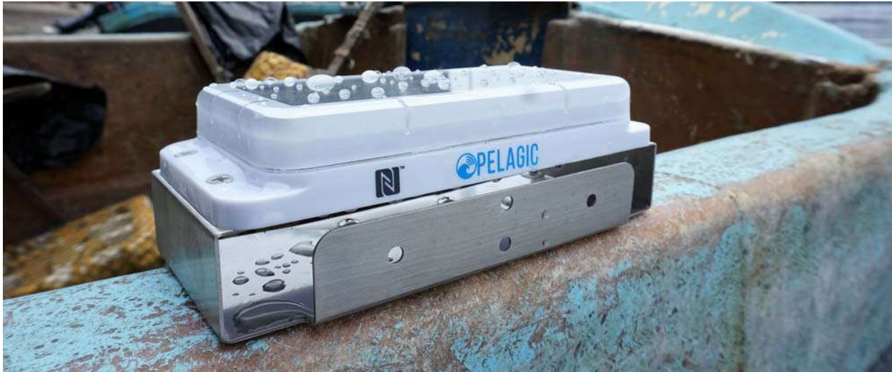
Figure 11. Pelagic Data Systems Solar Logger unit ( www.pelagicdata.com ).
