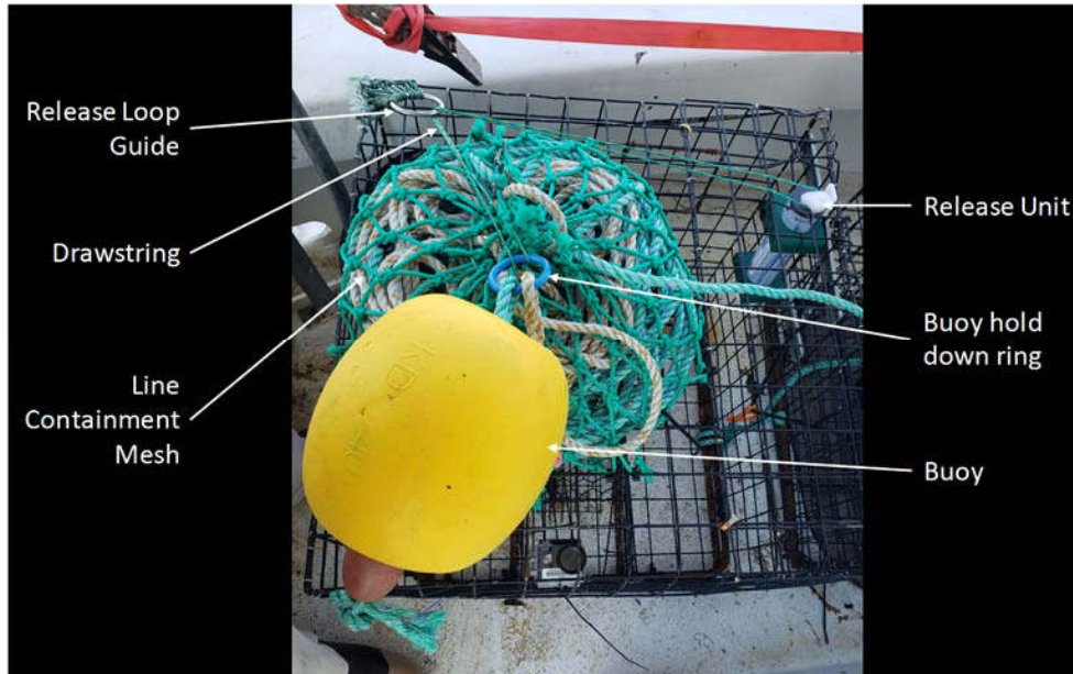
Figure 8. Longsoaker Guardian drawstring/mesh line handling system.
