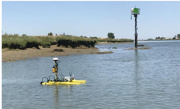
*USGS Autonomous Vessel Measuring at Flow Station 11455095
