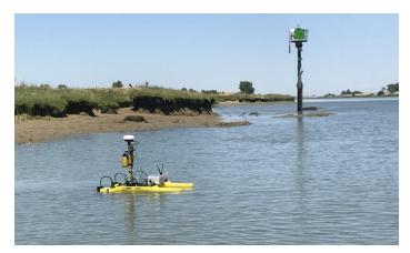
USGS Autonomous Vessel Measuring at Flow Station 11455095 in the Sacramento Deepwater Shipping Channel
