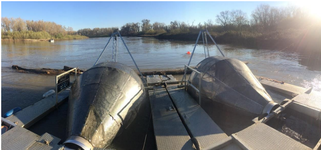
Figure 1. Rotary screw traps on the Sacramento River at Knights Landing.
