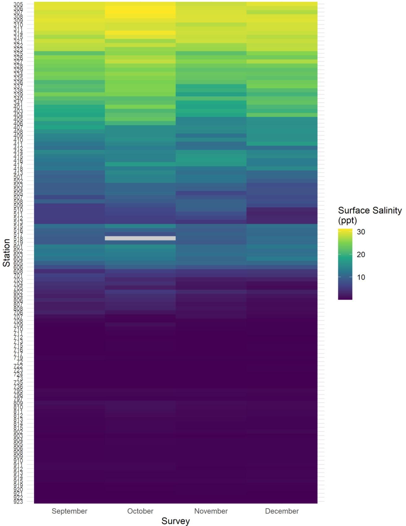
Figure 11. Heatmap of monthly surface water salinity (ppt) recorded during the 2022 FMWT season. White values indicate missing data. The low salinity zone (0.5-6 ppt, dark purple stations) stayed inland upstream of the confluence of the San Joaquin and Sacramento Rivers.
