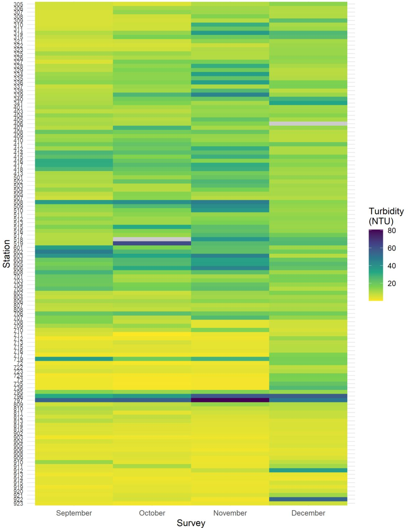
Figure 4. Heatmap of surface water turbidity (NTU) recorded during the 2022 FMWT season. White values indicate missing data. The northern part of the DWSC, northern Suisun Bay, and San Pablo Bay were the most turbid regions which varied among months.
