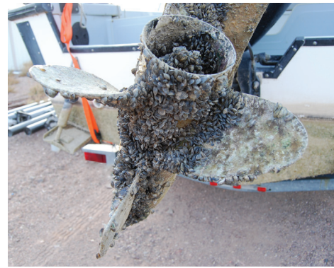
Quagga mussels attach to the hulls and propellers of recreational watercraft, impairing their operation and potentially moving with them to other waterbodies. Photo: National Park Service
