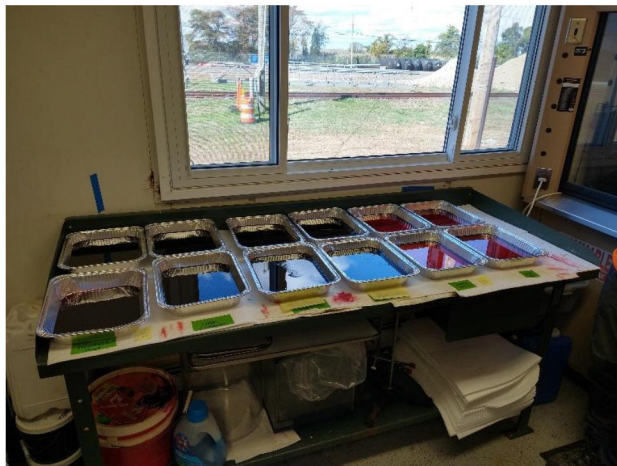
ASTM F726-17 tests in Ohmsett's chemistry lab
