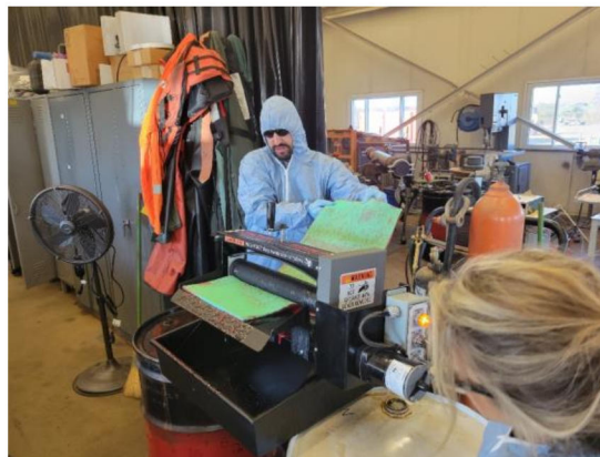
AquaFlex®'s wringer system for reusability tests
