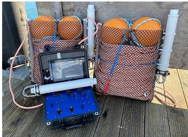
Figure 1. Deck box, acoustic transducer, and release bag with ARC-1XD release.
