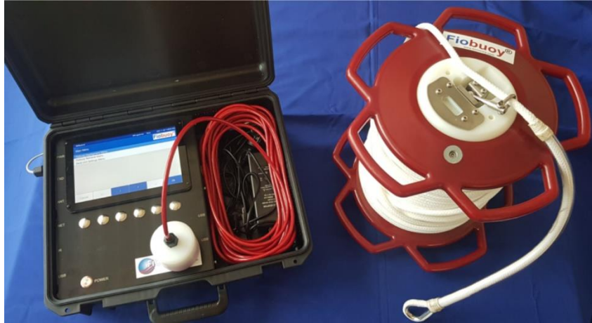
Figure 9. Deck unit, acoustic transducer and AC100 model Fiobuoy.
