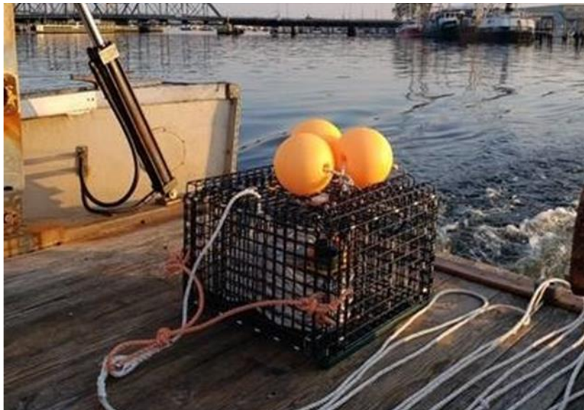
Figure 7. Release cage with bridle line attachment.
