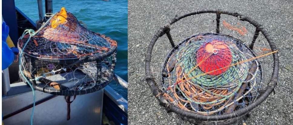
Figure 13. Guardian crab pot retrofit (left) and Guardian sled with 50 fathoms of line (right).
