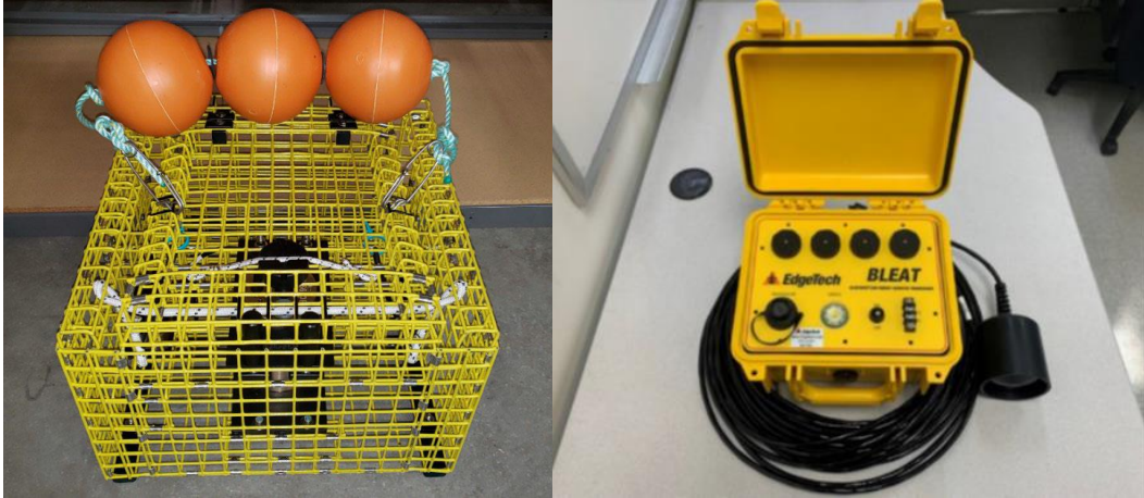
Figure 5. 22.5-in configured cage and BLEAT portable deck box with dunking transducer.
