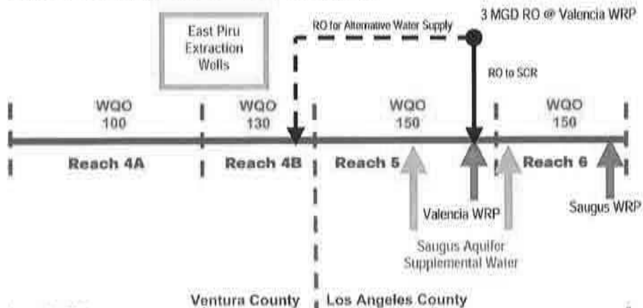
Figure 1a. AWRM Operation when SWP Cl \geq 80 mg/L
