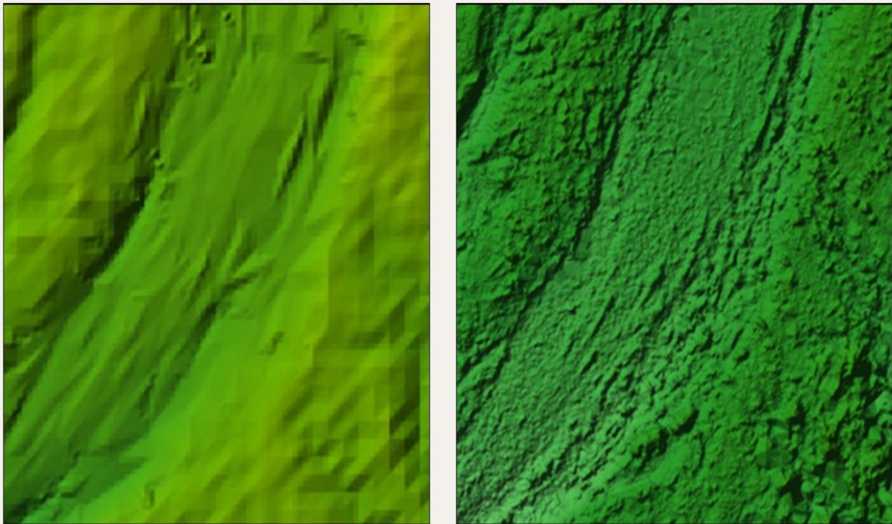
**Figure 11.** DTM generated from field survey points and 2005 3-m LIDAR (left) compared to 2018 0.25-m QL1 LIDAR (right).
