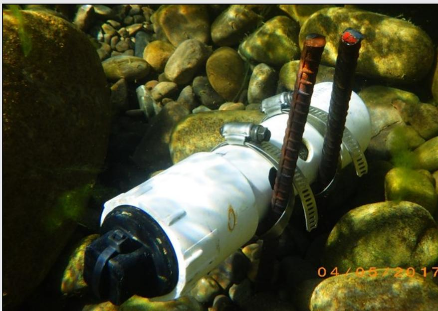
**Figure 2.** Pressure transducer installed in the stream bed to monitor water level.
