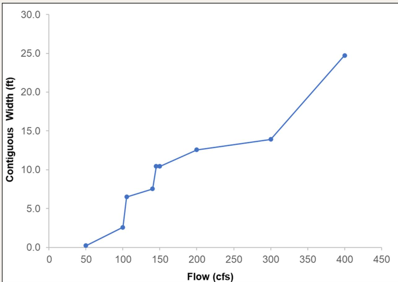
**Figure 12.** Flow versus contiguous width at the most depth-sensitive portion of the Ventura River study site.
