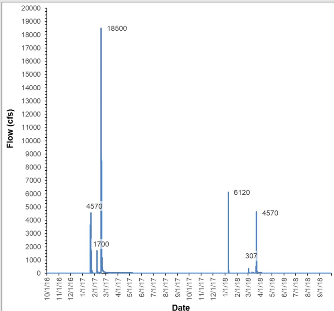
**Figure 3.** Flows recorded in the Ventura River at Foster Park (USGS 11118500) during water years 2017-2018.
