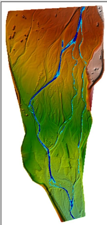
**Figure 5.** A digital representation of the depth-sensitive area of the Intermittent Reach displaying the three main distributaries.
