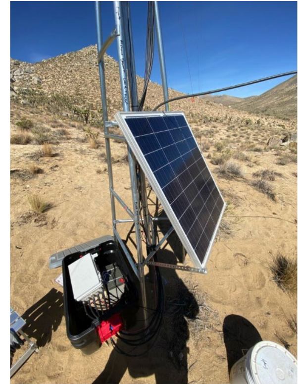
Motus avian monitoring unit installed at Frog Spring; Mojave Desert Springs Project
