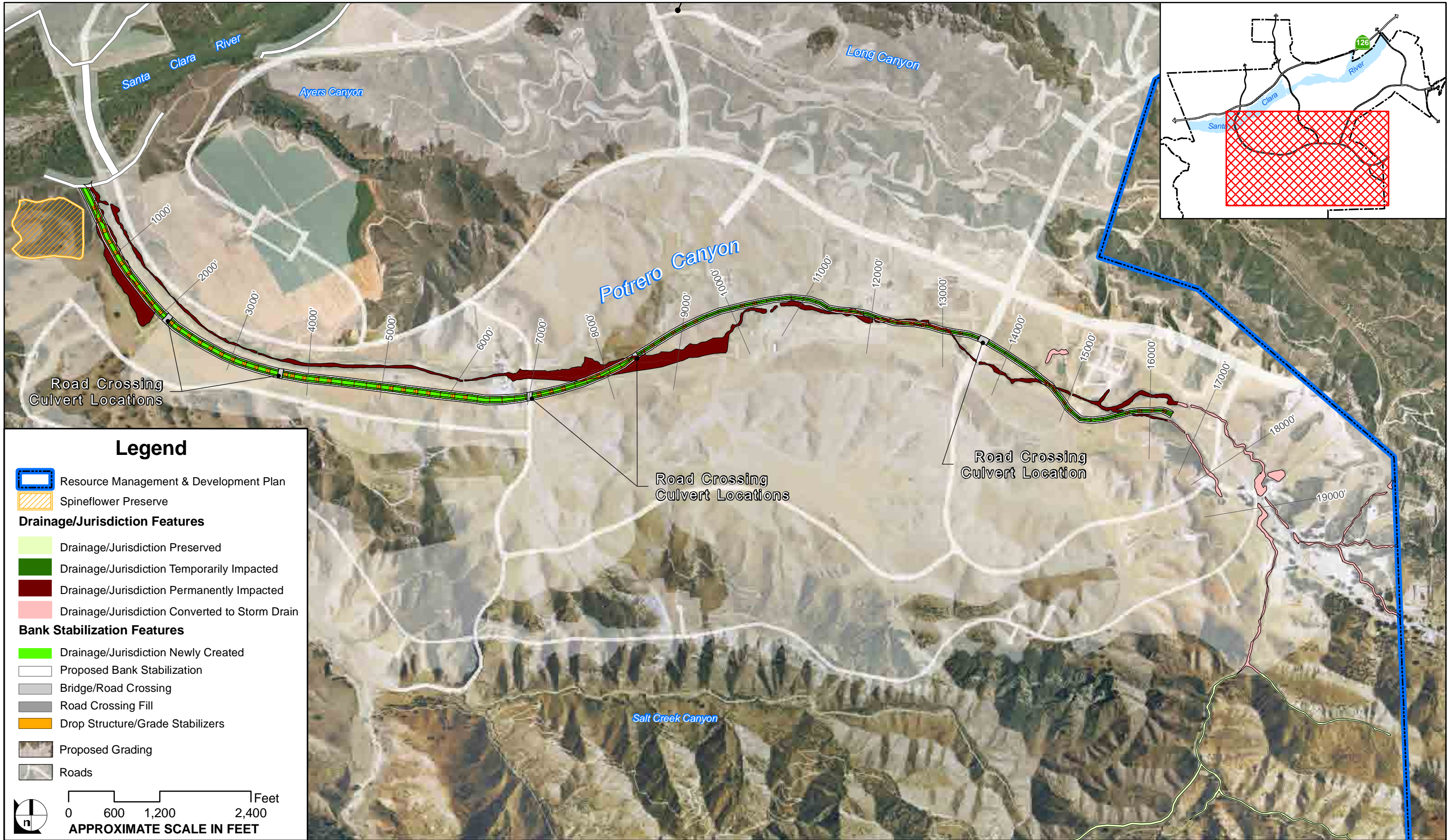
FIGURE 2.0-43 PROPOSED POTRERO CANYON DRAINAGE TREATMENTS
