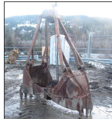
Figure 2. The 150-ft tall crane's grab dredge used for sediment removal.
