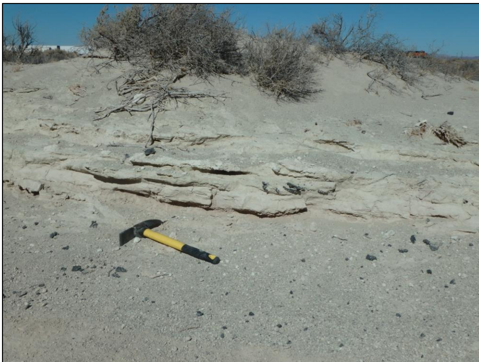
Figure 12. Quaternary clays (Qc) exposed in a shallow channel along National Trails Highway (Historic Route 66). Clay consisted of buff silt and clay deposits, massive to loosely bedded, with lenses of very fine-grained windblown sand and silt and scant igneous rock pebbles and small cobbles. View north.
