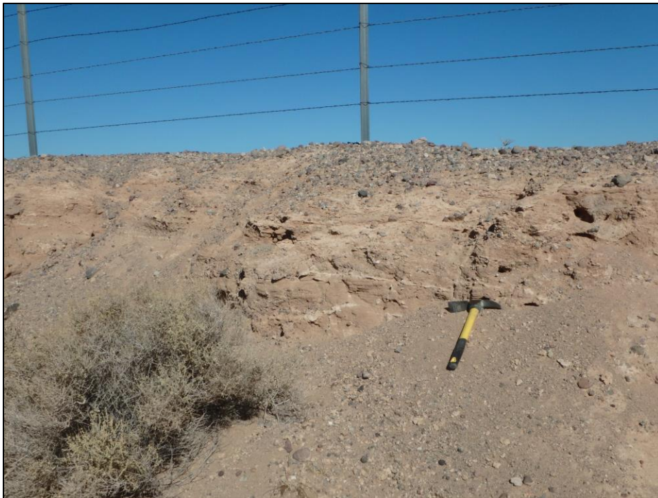
Figure 8. Quaternary older fan deposits (Qof) less than 1-foot below ground surface, showing very fine-grained sand and silt, poorly to moderately consolidated, and well sorted, with scant cobble-sized igneous rock clasts. View west.
