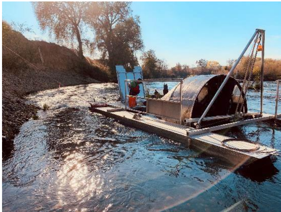
Figure 6. Photo of a rotary screw trap in the fishing position in the SJRRA during a routine trap check. Photo credit: Reclamation.
