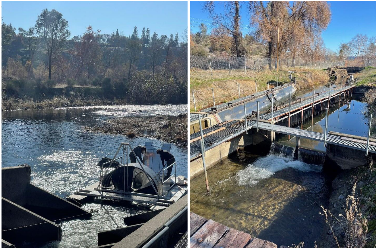
Figure 1. Photos taken in December 2022 of the rotary screw trap (left) and the off-stream diversion fish screen (right) operated by CDFW at the nearby Parrott-Phelan Diversion Dam. Photo credit: USFWS.
