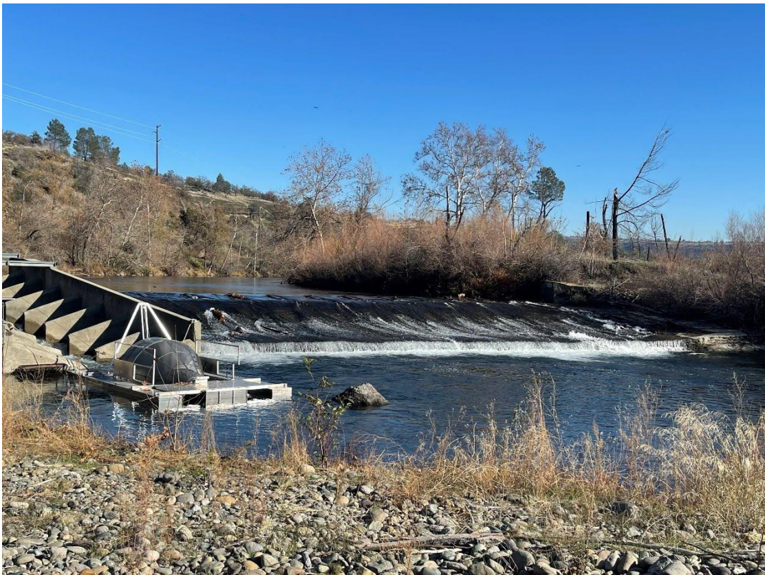
Figure 4. Photo taken in December 2022 of the rotary screw trap operated by CDFW at the Parrott-Phelan Diversion Dam. Photo credit: USFWS.
