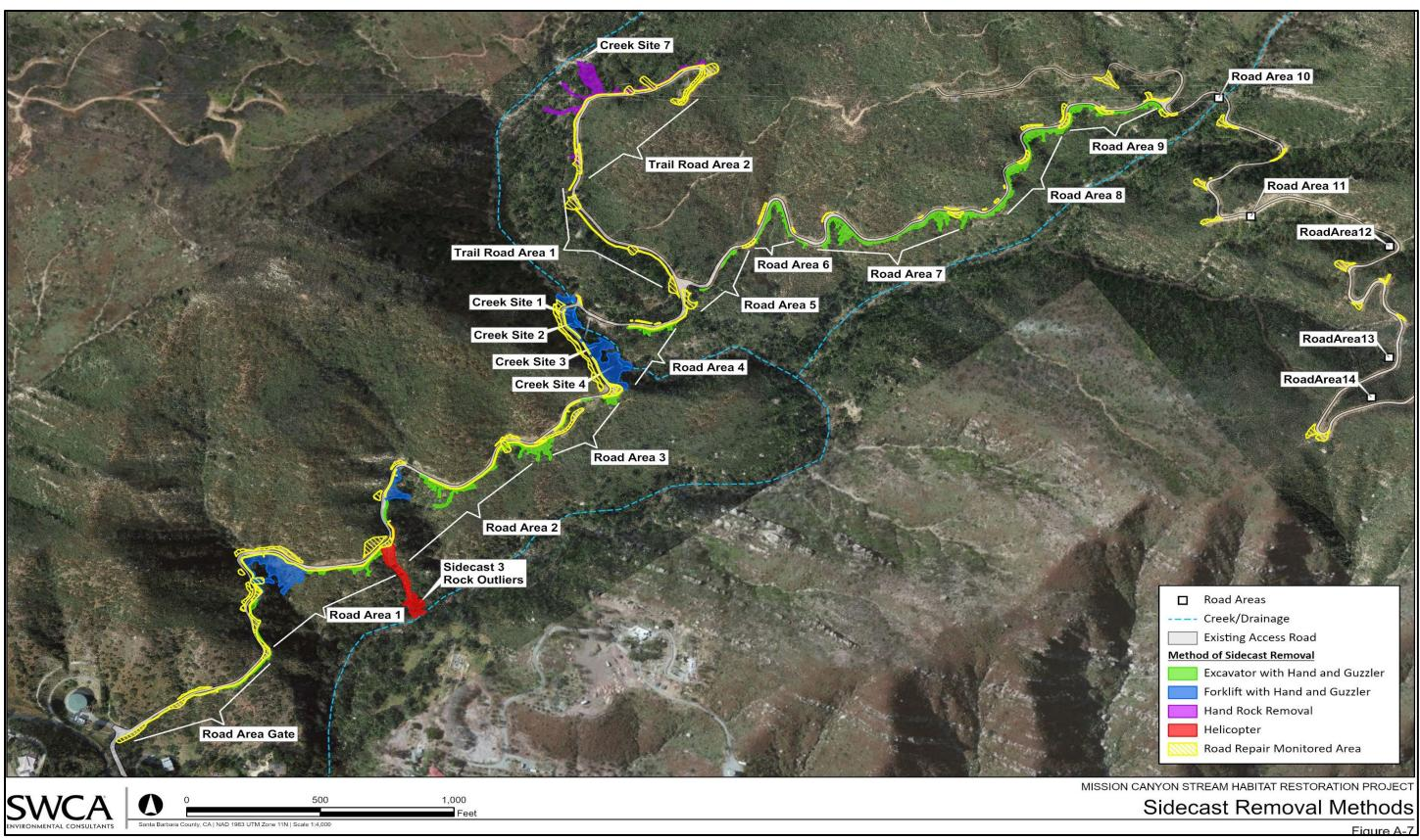
Figure 4. Project area with sidecast removal techniques.
