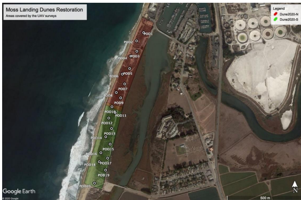
Figure 25. UAV Study area. The colored polygons outline the two separate survey areas. The label identifies the GCPs used for the surveys.
