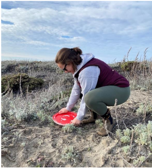
Left: Bucket lids being put on ground control points before the UAV /survey. Right: UAV departing Moss Landing Marine Labs for survey at SRSB
