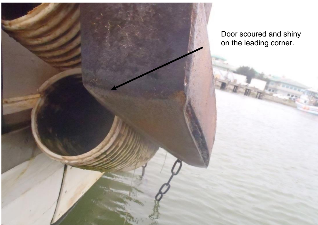
Figure 9 Trawl door showing evidence of minimal contact with seafloor (Wick et al. 2014) (Photo credit: NOAA Fisheries)
