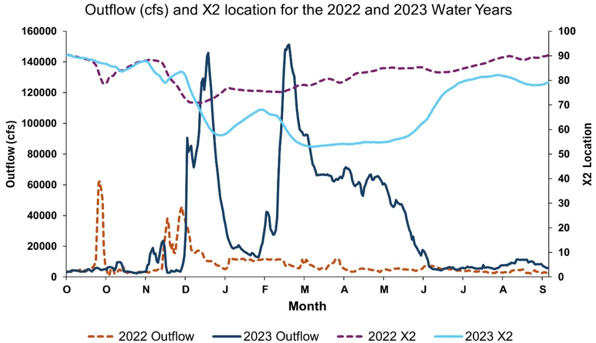
Figure 3. Line plot showing daily net Delta Outflow values and X2 location for water years 2022 and 2023. Outflow is displayed on the left y-axis in cubic feet per second (cfs). X2 location is conveyed on the right y-axis as river kilometers upstream from the Golden Gate Bridge. Months are shown on the x-axis starting with October and ending with September.
