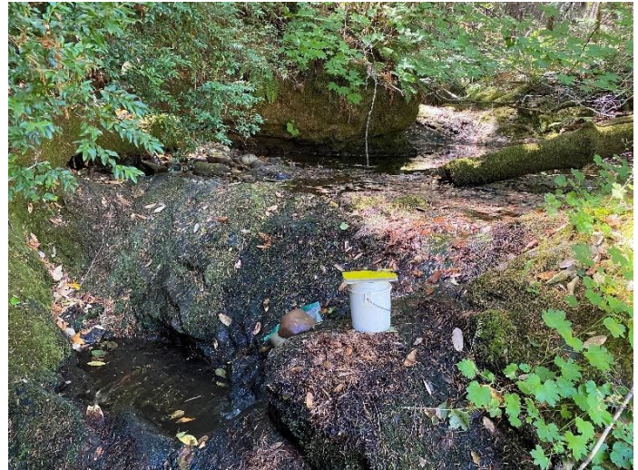
Anderson Creek volumetric streamflow measurement site. Dissolved oxygen is measured in the pool above the cascade.
