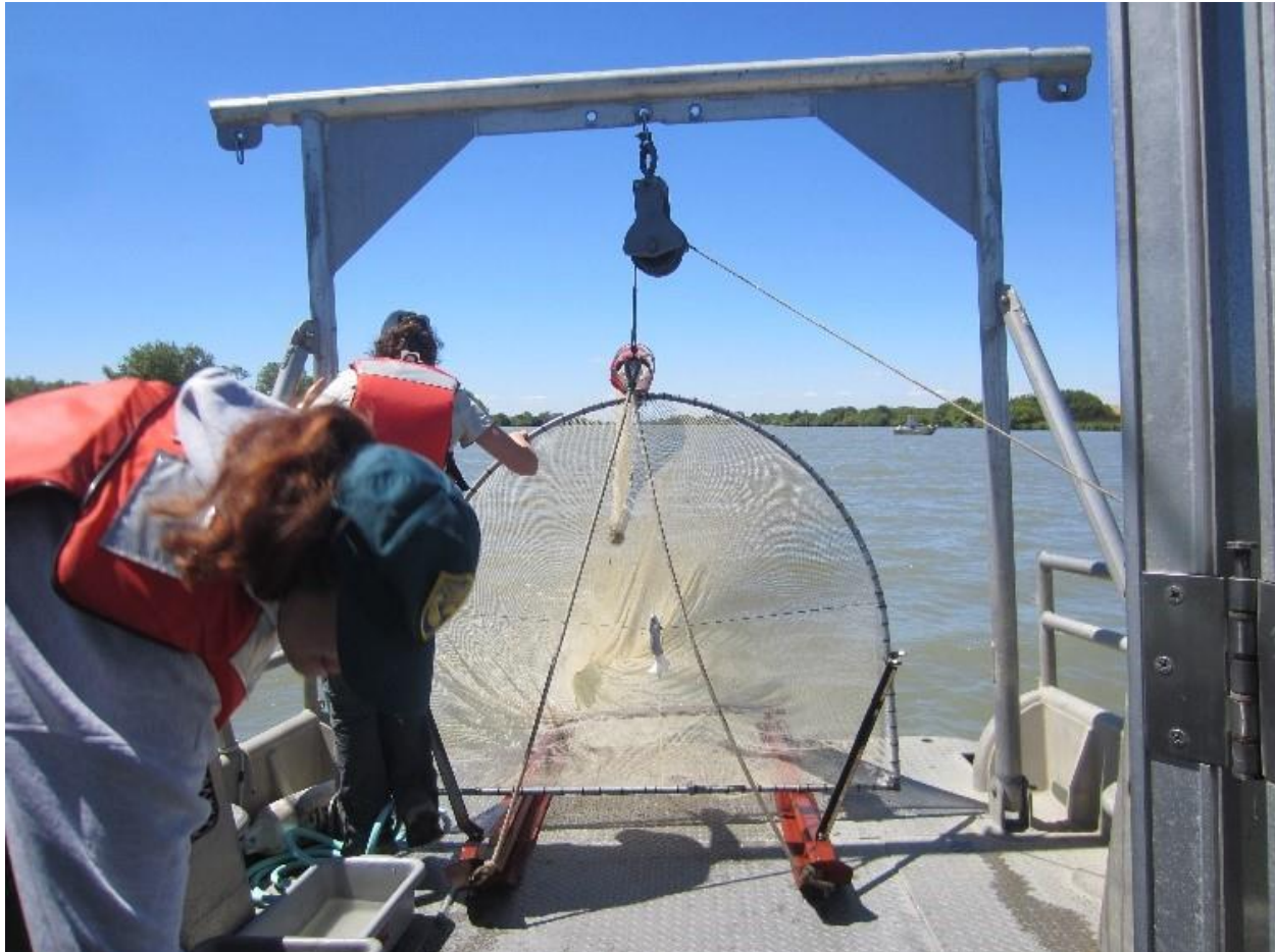
Figure 2. Towntet ready for deployment with meso-zooplankton (Clark-Bumpus) net mounted on top, and flowmeter attached to the center of the townet.
