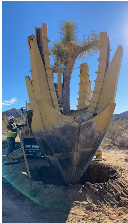
Figure 2. A salvage tree being removed from the ground using a tree spade (Photo credit: National Park Service).
