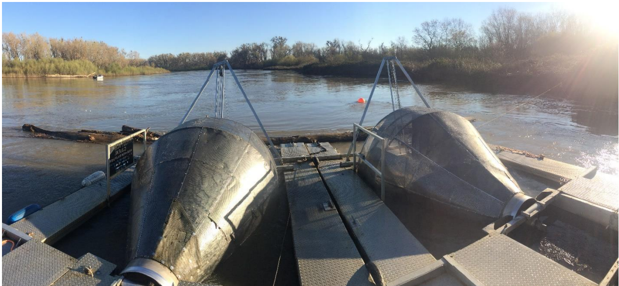
Rotary screw traps on the Sacramento River at Knights Landing.
