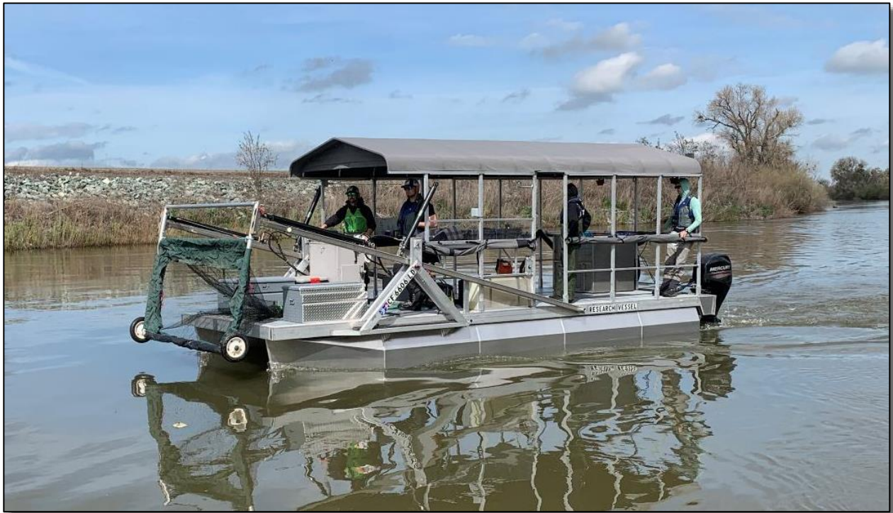
Figure 1: Aquatic Habitat Sampling Platform (Cramer Fish Sciences)
