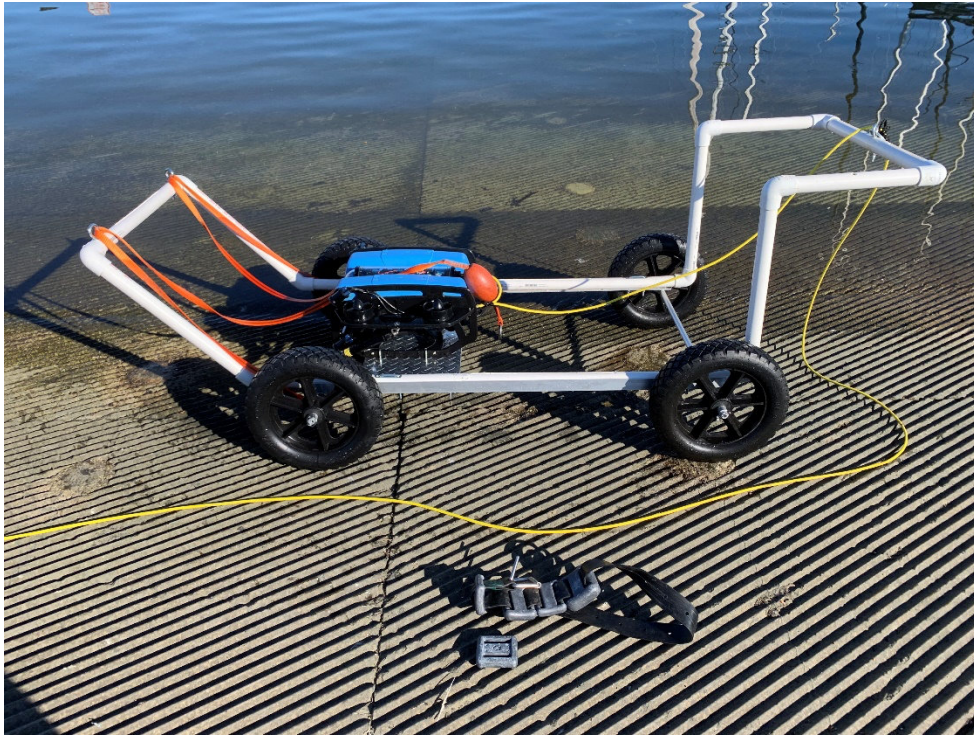
Figure 4-3: SBSR ROV and Tow Vehicle for Bottom Surveying
