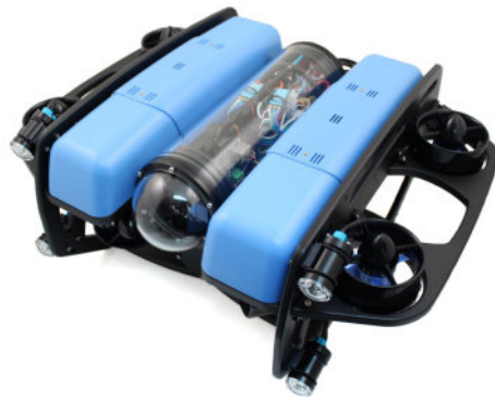
Figure 4-2: SBSR's BlueROV2 Heavy Configuration ROV
