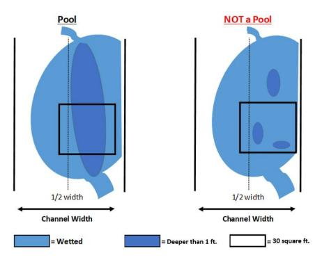
Figure 39. Top view of two habitat units, where the one on the left is a pool because it is greater than 1-ft. in depth for at least as long as the wetted width. The habitat unit on the right does not meet the minimum pool metrics because it only has a few isolated spots where the depth is greater than 1-ft. (source: Sea Grant 2022).
