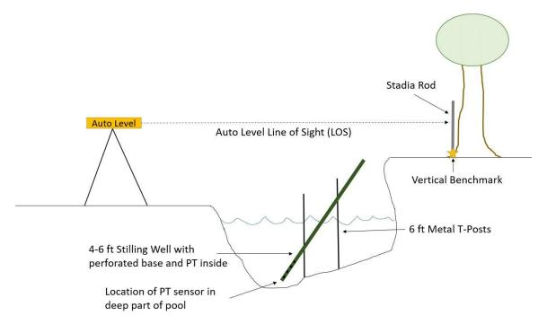
Figure 15. Ensure that the VBM and PT pool are visible from the location of the auto level and that the VBM is lower than auto level line of sight.
