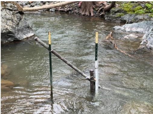
Figure 10. A 3-4-ft housing with DO logger inside is attached to a T-post next to staff plate (right side of photo). The 6-8-ft PT housing is affixed diagonally across both T-posts in the pool.
