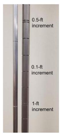
Figure 19. Hexagonal portion of the top-setting wading rod measures depth and has graduations of 0.10-ft.
