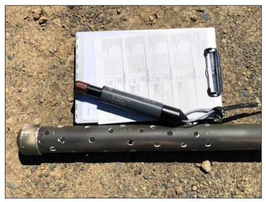
Figure 5. Dissolved oxygen logger with anti-fouling guard covering the sensor cap. Cable is attached to the cap of the logger. Also shown is the perforated bottom of a camouflaged housing.
