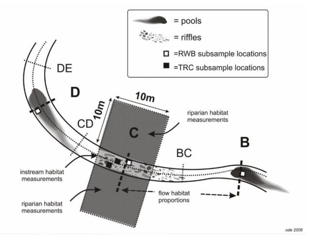
Figure 37. The section of the standard reach showing the appropriate positions for collecting riparian habitat and flow habitat proportion measurements. Also shown here is the human-influence zone corresponding to the area within 10m of the wetted width (i.e., zone "C").
