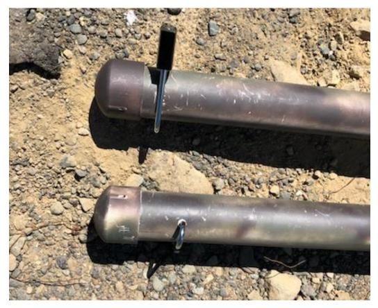
Figure 6. Camouflaged housings with caps and padlocks with holes drilled through the top. The DO loggers are hung with cable inside the housings and attached to padlock clasps for easy retrieval.
