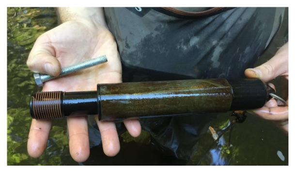
Figure 32. Example of moderate biofouling accumulated on a DO logger.
