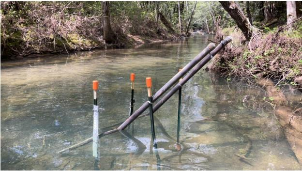
Figure 7. Six-ft PT housing installation.
