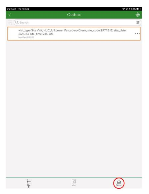
Figure 24. Screenshot of the CEMAF Hydrology and Water Quality survey Outbox page. Note that there is one Site Visit that needs to be uploaded (highlighted by the orange rectangle). Use the "send" button to upload the survey to AGOL.
