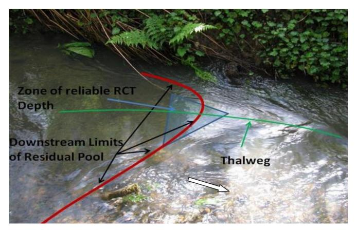
Figure 30. Riffle crest in small, confined stream where the RCT is easy to locate. (Reprinted from Rossi 2012).
