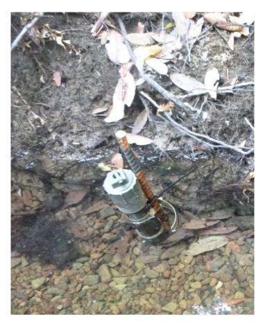
Figure 9. Pressure transducer with 16-in HOBO® housing installation affixed to rebar. Photo taken at end of gaging season (October). PT should be fully submerged during installation.
