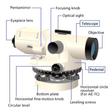
Figure 14. Diagram of the various components of an auto level (reprinted from California State Parks, 2019).
