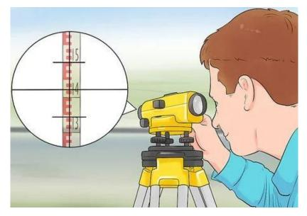
Figure 17. Example of how to use the auto level crosshairs to take a measurement on the stadia rod. Ensure that you use the middle crosshair when taking a reading. For example, in this image, the reading would be 14.2 ft (reprinted from WikiHow article by Kamran, 2024).
