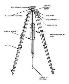
Figure 13. Diagram of a surveyor's tripod (reprinted from California State Parks, 2019).
