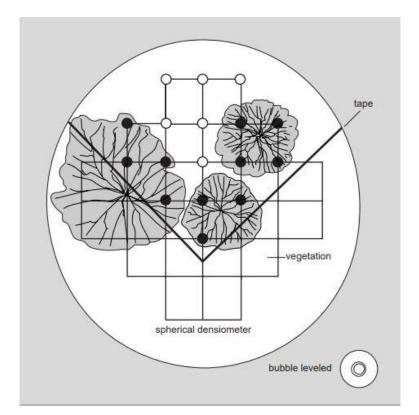
Figure 38. A concave spherical densiometer with bubble level, tape, and 17 points of observation. Closed circles represent line intersections counted in measurement of canopy closure (11 out of 17 points) (Reprinted from Fitzpatrick 1998)
