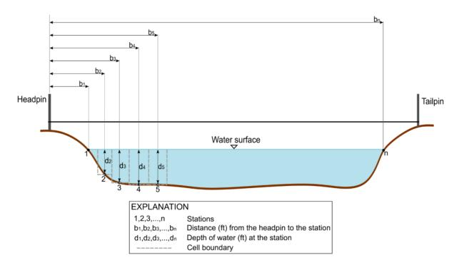
Figure 22. Cross section showing vertical measurement cells and the distances used to determine cell width using the mid-section method. Headpin, tailpin, and measuring tape are indicated over the cross section. Figure adapted from Turnipseed and Sauer (2010).
