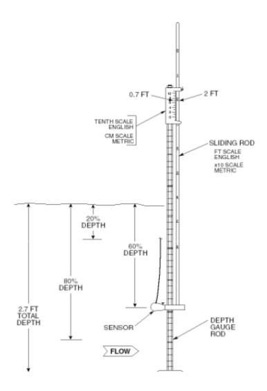
Figure 21. Diagram showing velocity measurement locations at 0.2 (20%), 0.6 (60%) and 0.8 (80%) depth within a channel, and how these are measured using a wading rod and current meter (Nolan and Shields, 2000).
