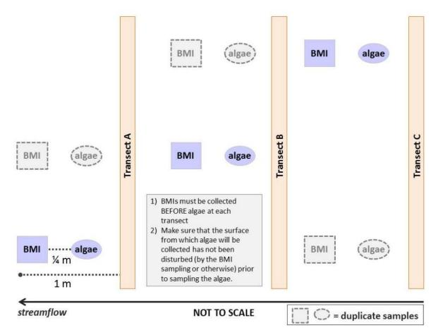
Figure 35. Sampling array for collection of BMIs, algae, and duplicate samples (outlined with dashed lines) for each assemblage. Figure reproduced from SWAMP SOP for the Collection of Field. Note that CEMAF does not collect algae at this time. For convenience, only Transects A through C of the sampling reach are shown, but the same pattern of placement should be rotated across all 11 transects.
