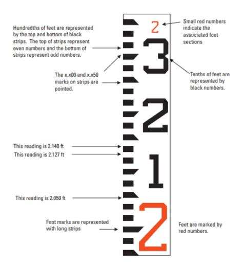
Figure 16. Staff plates and stadia rods allow you to measure to the nearest thousandth of a foot. The depiction of a staff plate or stadia rod above indicates how to properly interpret measurements to the thousandths of ft (reprinted from U.S. Geological Survey, 2010).
