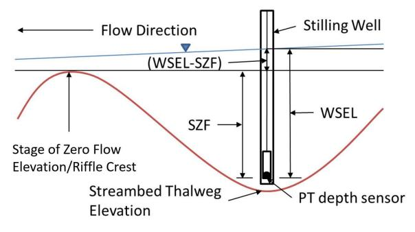
Figure 29. Stage of Zero Flow (SZF) diagram. The blue line represents the water surface (reprinted with permission and minor modification: Cowan, 2018).
