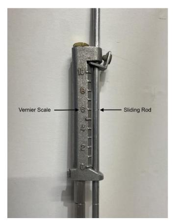
Figure 20. Vernier scale and sliding rod aligned for measuring flow at 0.6-ft depth.
