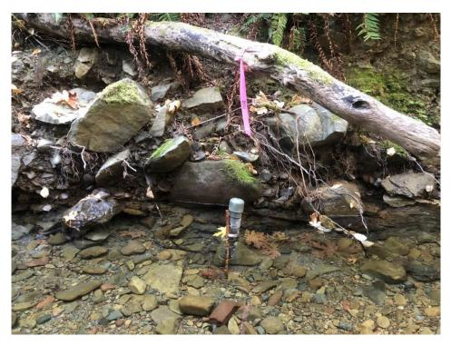
Figure 11. A 16-in PVC housing affixed to rebar. This photo was taken at retrieval during baseflow conditions. Housing should be fully under water at deployment.
