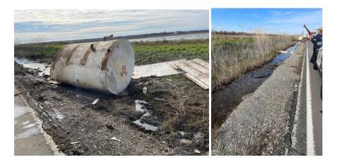
25-0767: Jet fuel, Richvale, Butte County – NFRT members responded to a report of a fuel tanker carrying 450 gallons of Jet A Fuel and 400 gallons of water overturning, releasing its contents. The fuel and water leaked into a six-inch-deep ditch on the side of the road. NFRT concluded that the ditch was not hydrologically connected to state waters and Butte County Environmental Health coordinated the cleanup. No wildlife impacts were observed, and no state waters were impacted.
