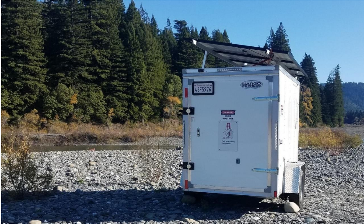
11.) Cargo trailer with mounted solar panels at Main Stem Eel River sonar site.
