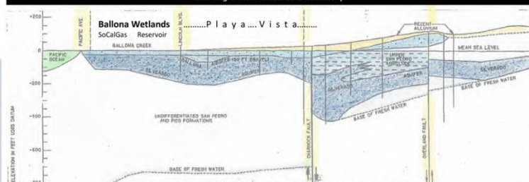
Figure 7. Generalized E-W Hydrogeologic Cross Section (Modified after Cal. Dept. Wtr. Res., 1961 & CDM, 1998)
