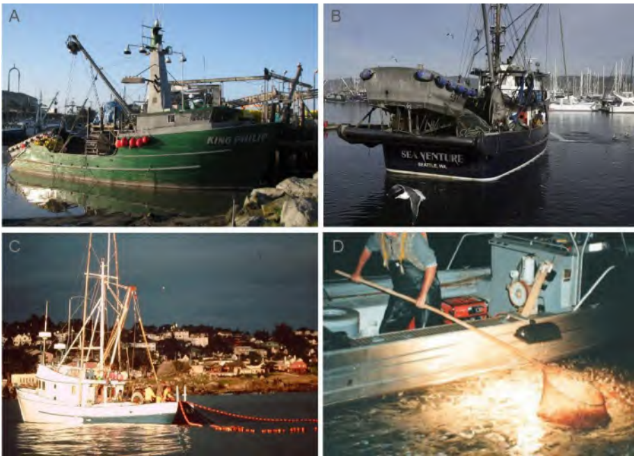
Figure 2-4. Vessels equipped with (A) purse seine gear (B) drum seine gear (C) lampara gear (D) brail/dip net gear (Photo Credit: CDFW).
