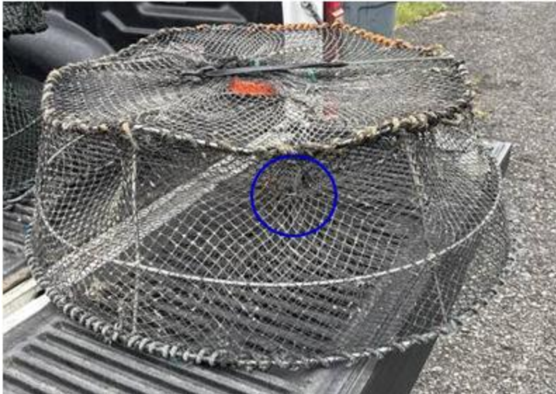
Figure 1. Image of a single-chambered coonstripe shrimp trap showing woven mesh and escape opening shown in blue circle. Photo credit: T. Wakefield.
