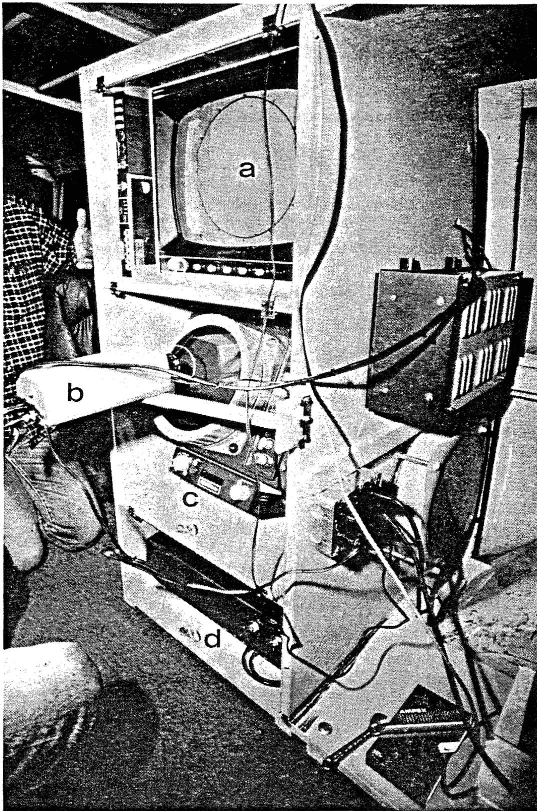
Figure 6. Interior of utility van showing monitoring equipment: a) video monitor, b) TV camera, c) radar (PPI) screen, d) video recorder.
