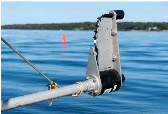
Figure 4 Vessel system. Transducers on a pole mount configuration (LEFT) cabled to the transceiver box (RIGHT). The transceiver box manages all communications between the chartplotter and seafloor gear and with any shoreside databases (RMWHub or EarthRanger).
