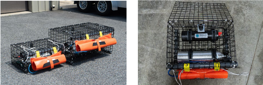
Figure 2 RISER MTA seafloor recovery systems in two sizes (LEFT) and view of components inside mesh frame (RIGHT).
