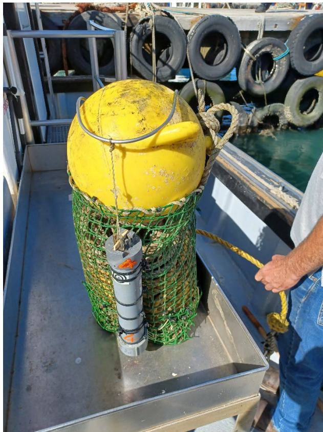
ARC-2 on the side of a bag custom designed by SA Sensational Seafood (South Africa) for hauling heavy trawls in the shallow (~10-20 fathom) but rough waters near Cape Town. The ARC-2 shown here has experienced approx. 18 months of near continuous service.
