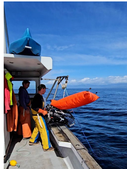
Figure 1 RISER MTA seafloor recovery system ready for deployment (LEFT) and recovered at surface ready for hauling (RIGHT).
