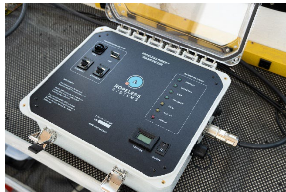
Figure 4 Vessel system. Transducers on a pole mount configuration (LEFT) cabled to the transceiver box (RIGHT). The transceiver box manages all communications between the chartplotter and seafloor gear and with any shoreside databases (RMWHub or EarthRanger).
