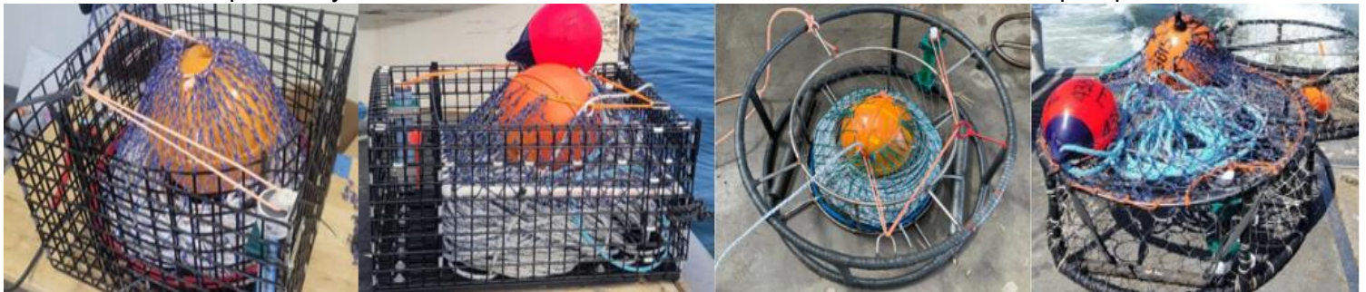
Figure 2. Guardian Inshore Sled (left), Mid-water Sled (middle left), Crab Pot Sled (middle right) and Trap-Top Retrofit (right).
