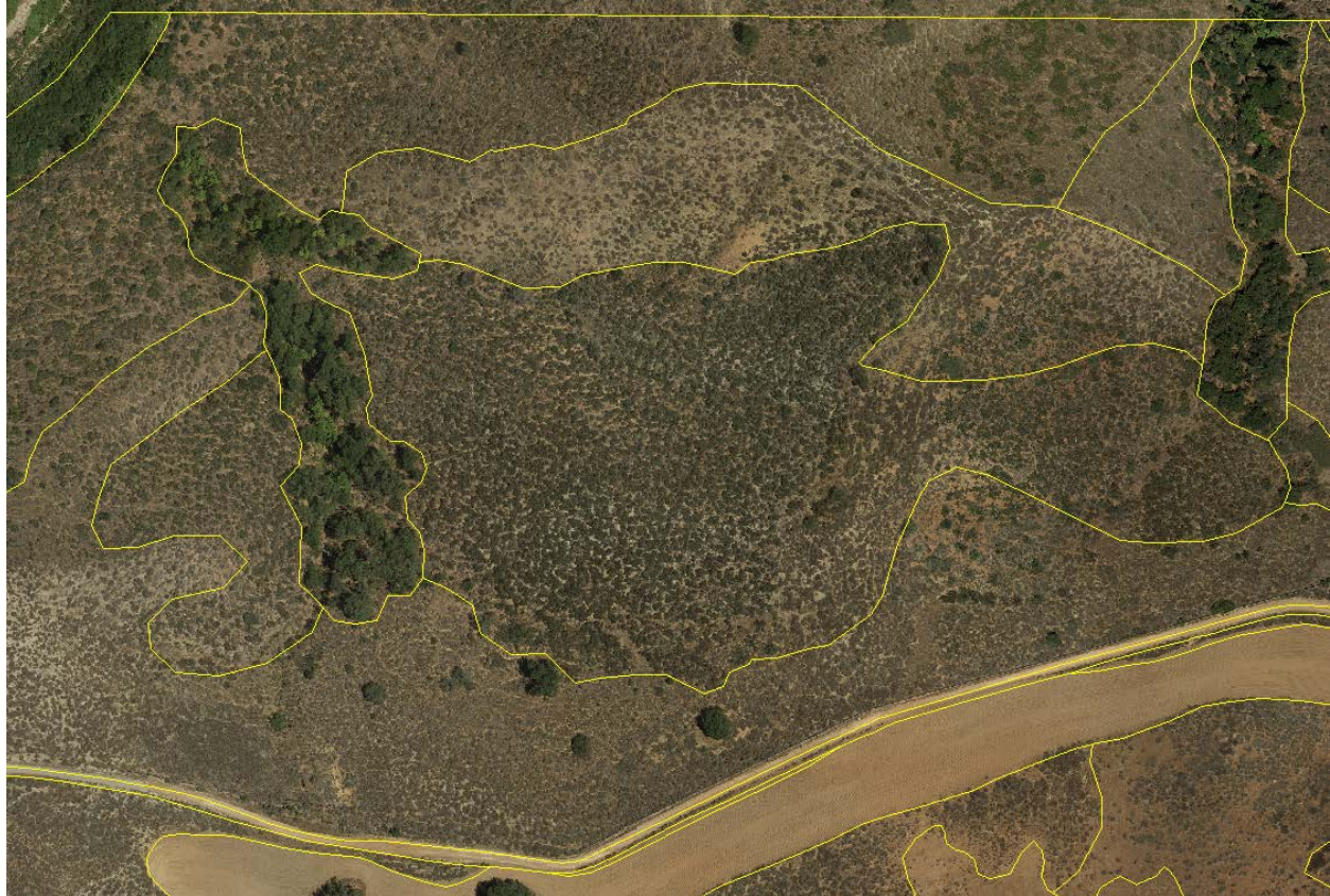
Figure 3-1. Example of photo-interpretation polygon creation conducted at a 1:2,000 scale.
