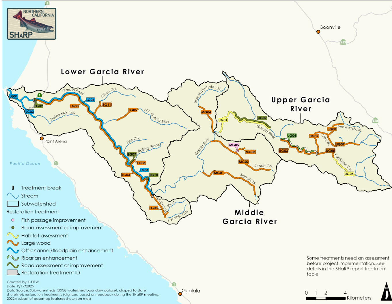
Figure 46. Restoration treatment map for the Lower Garcia River, Middle Garcia River, and Upper Garcia River HUC 12 subwatersheds for the Mendocino SHaRP. Treatment breaks delineate individual treatment extents when those adjacent were the same type. See Tables 27–29 for treatment details.
