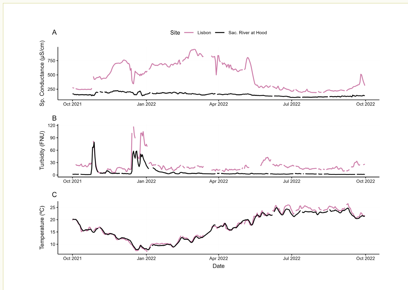
Figure 4. Time-series plots for specific conductivity (a), turbidity (b), and water temperature (c) at Lisbon Weir in the Yolo Bypass and Hood Station in the Sacramento River. The two continuous monitoring stations used in this report experienced several probe outages, scheduled maintenance, and unforeseen issues, resulting in data gaps.
