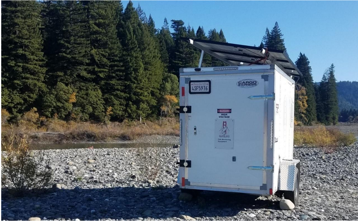
18.) Cargo trailer with mounted solar panels at Main Stem Eel River sonar site.
