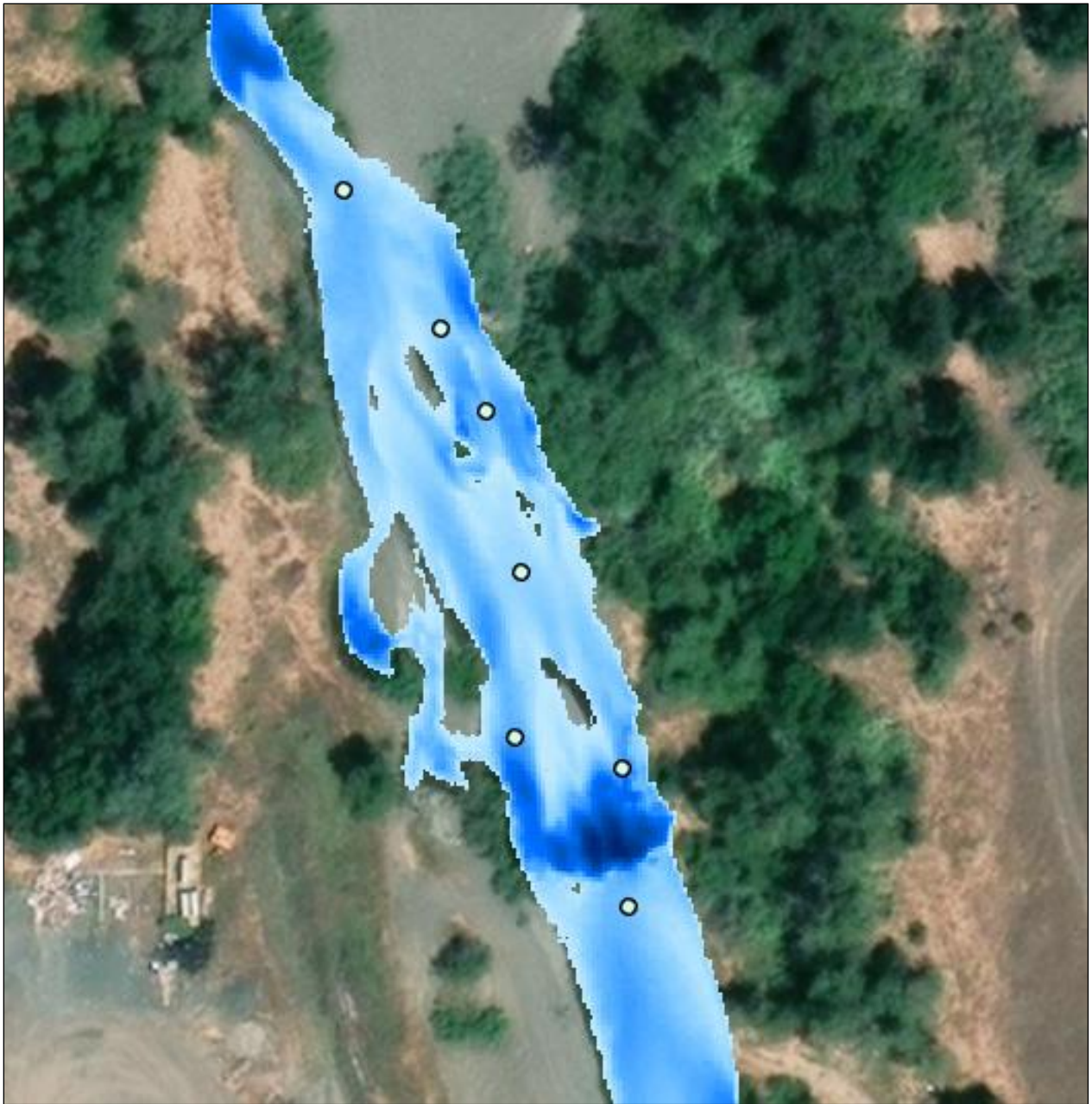
Figure 18. Field validation points collected along Kelsey Creek over the water depth raster simulated flow exported from HEC-RAS.
