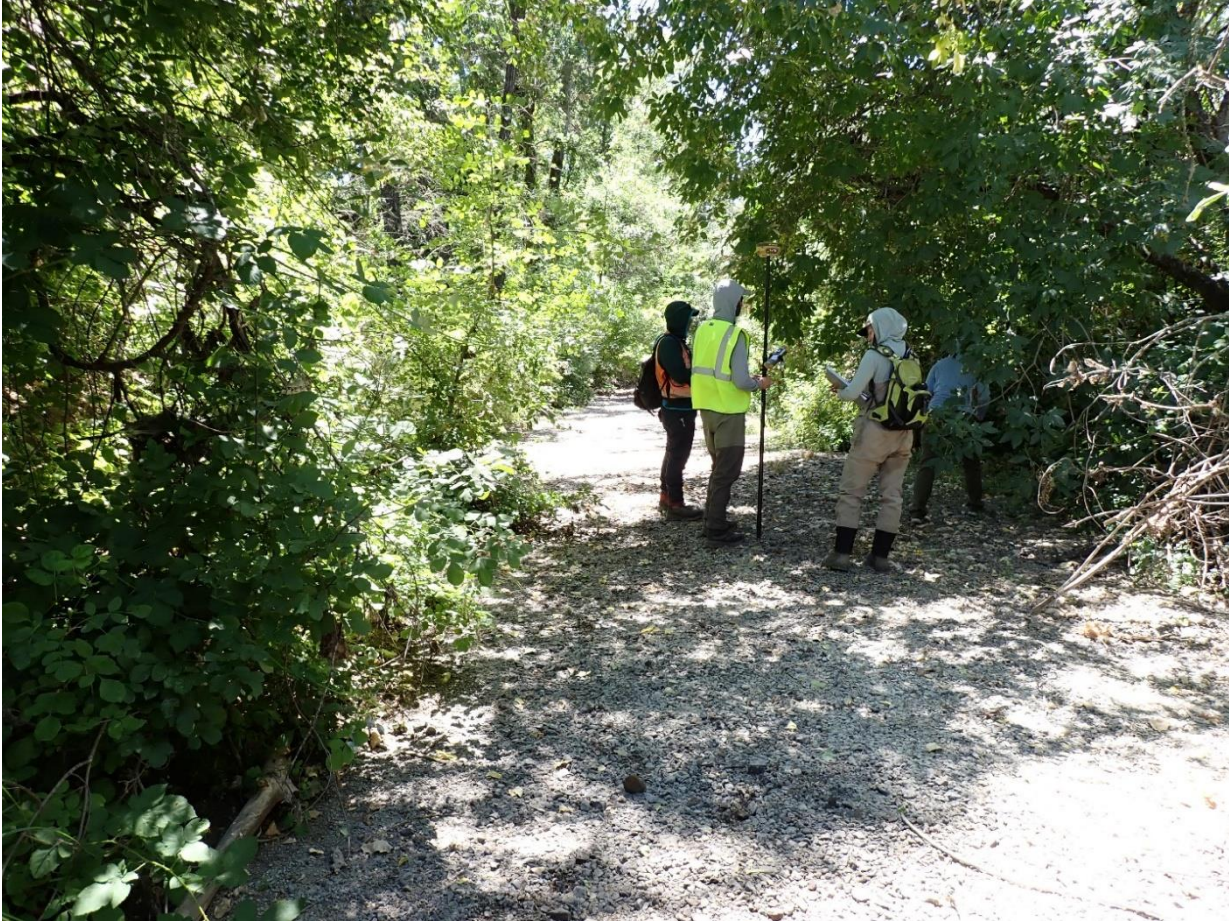
Figure 7. CDFW staff collecting location and elevation data under vegetation within Adobe Creek using an RTK-GPS unit.
