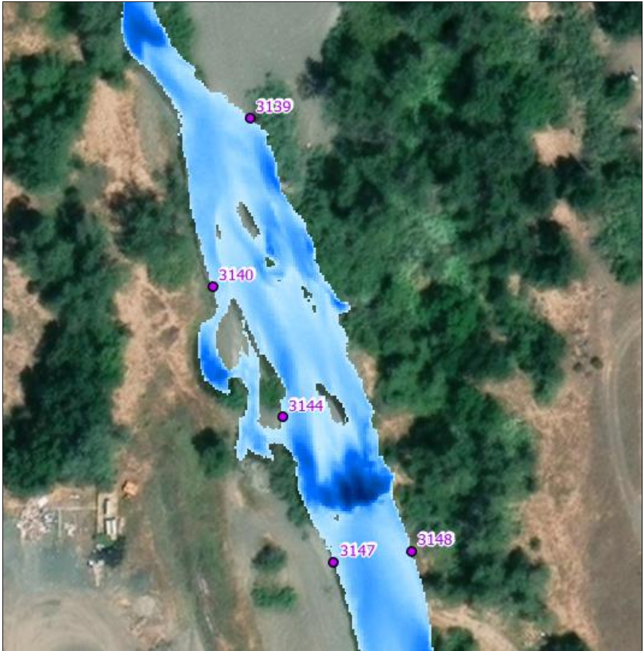
Figure 17. Water's edge water surface elevation points collected along Kelsey Creek over the water depth raster simulated flow exported from HEC-RAS. Discharge was collected along a transect between points 3147 and 3148.
