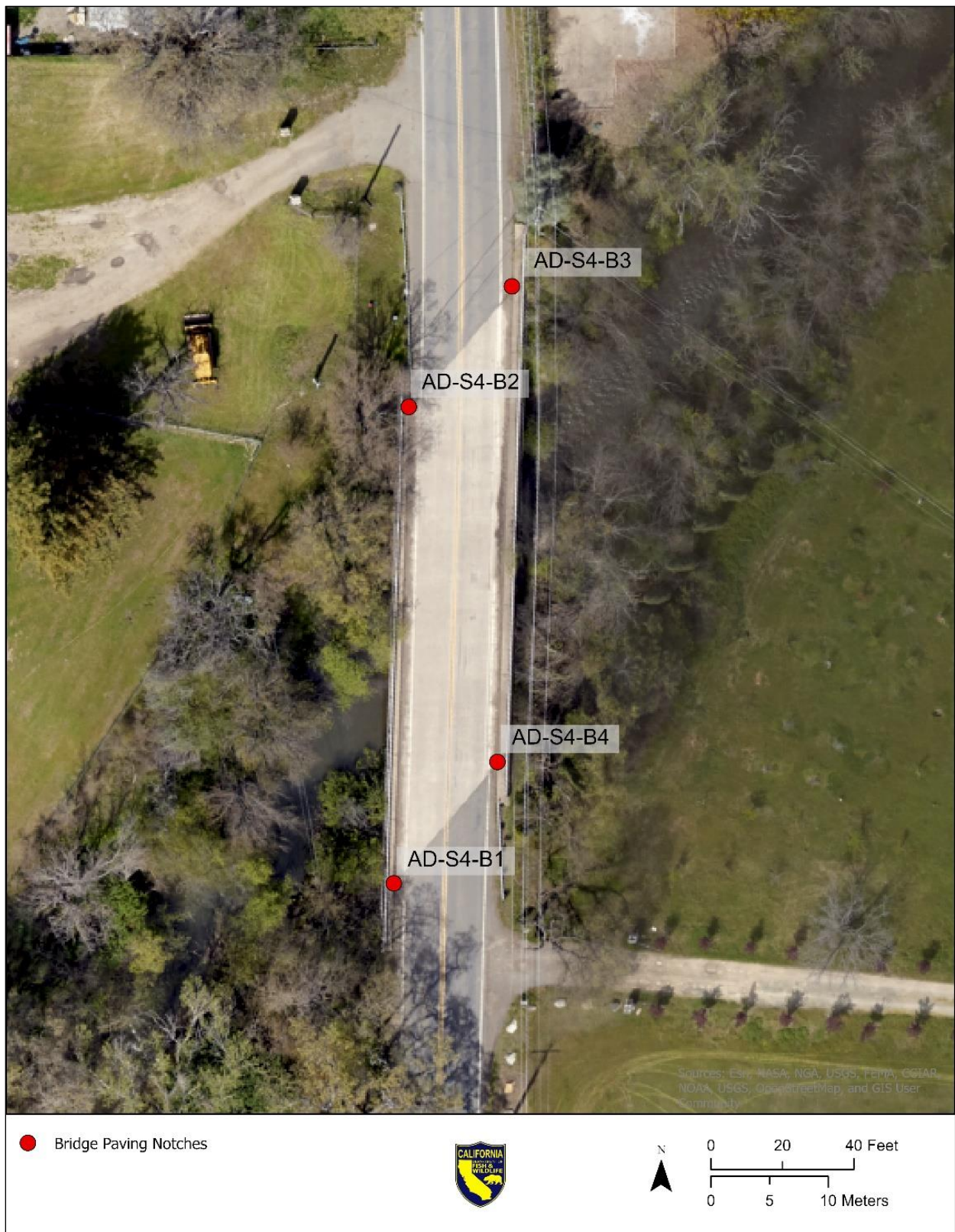
Figure 13. View of survey points at bridge paving notches at Soda Bay Road bridge crossing Adobe Creek.
