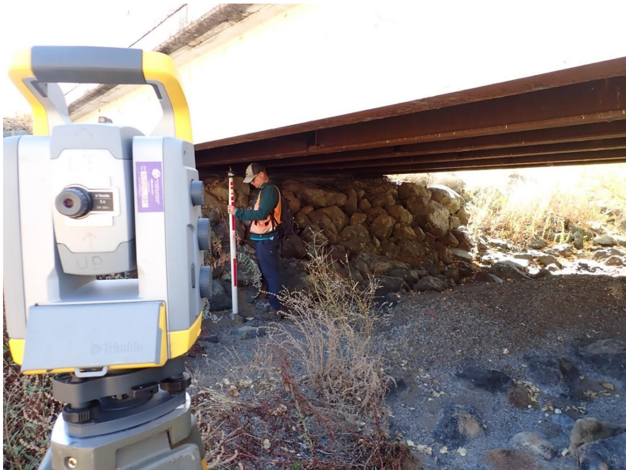
Figure 6. CDFW staff collecting location and elevation data under a bridge on Manning Creek using a total station.
