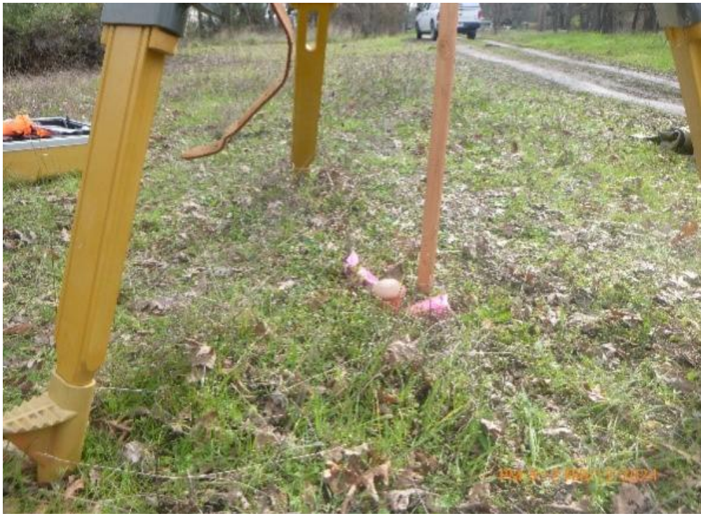
Figure B-2. Close-up view of a tripod for an RTK-GPS base station positioned over a ground control point.
