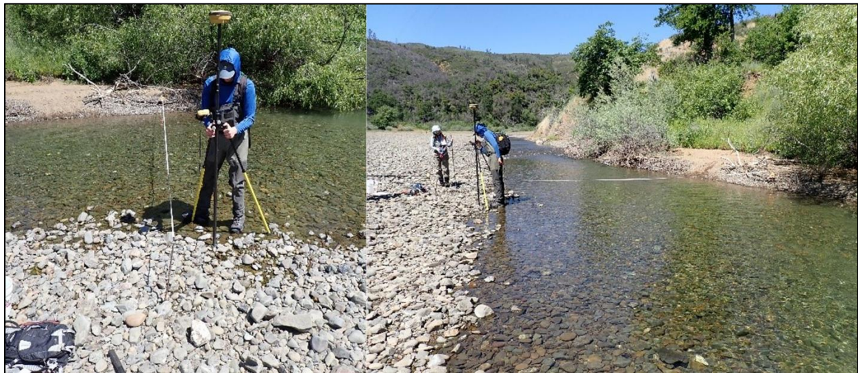
Figure C-6. CDFW field staff measuring water surface elevation and discharge on Scotts Creek near Cow Mountain Recreation Area, May 2024.
