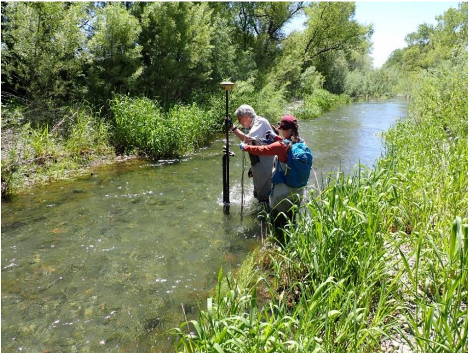
Figure D-6. CDFW field staff measuring depth, velocity, and GPS coordinates on Middle Creek near the confluence with Scotts Creek, May 2024.
