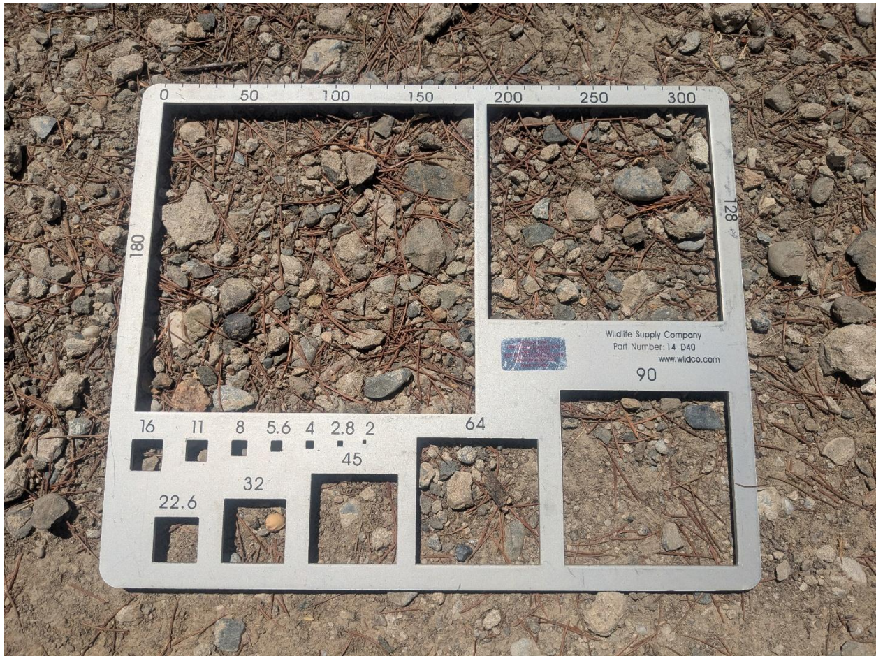
Figure E-2. Image of gravelometer used to conduct pebble count surveys. Numbers adjacent to each square opening indicate the particle size class (in mm) for that bin.
