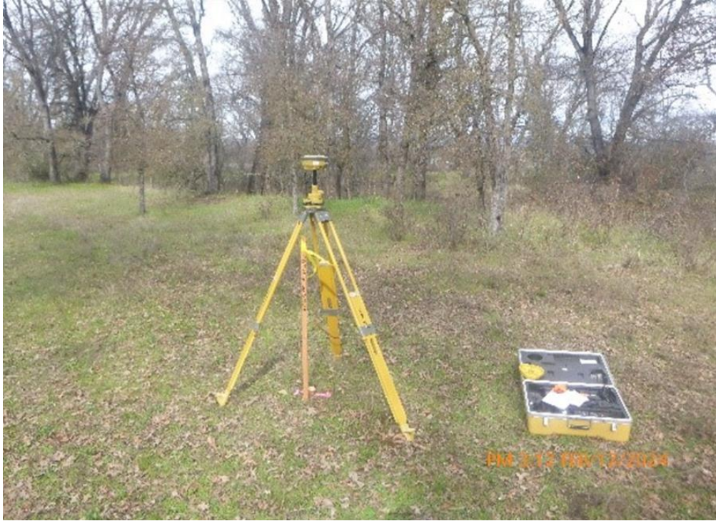
Figure B-1. Survey setup showing a tripod for an RTK-GPS base station positioned over a ground control point.
