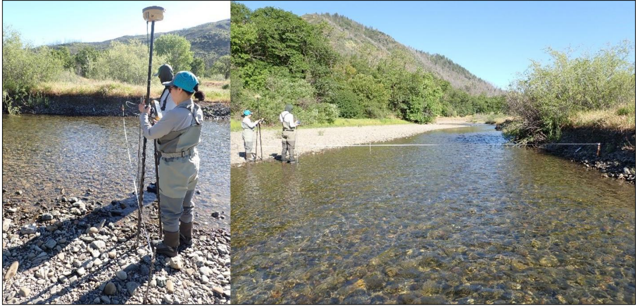
Figure C-5. CDFW field staff measuring water surface elevation and discharge on Middle Creek near Elk Mountain Road, May 2024.
