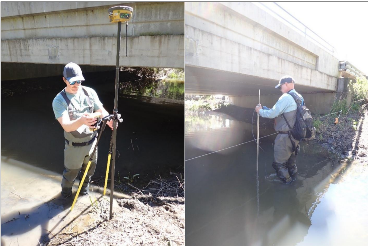
Figure C-2. CDFW field staff measuring water surface elevation and discharge on Cole Creek near Soda Bay Road, April 2024.
