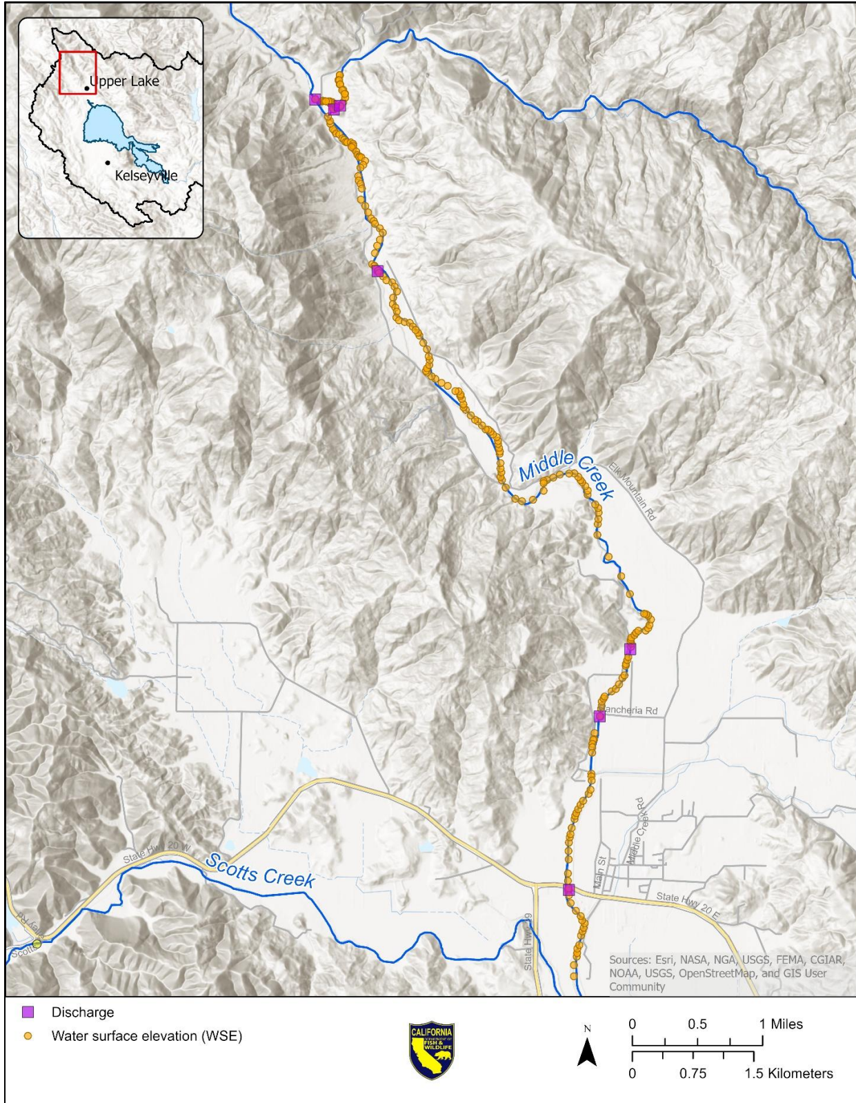
Figure C-10. Locations of water surface elevations (orange circles) and discharge measurements (purple squares) collected on Middle Creek.
