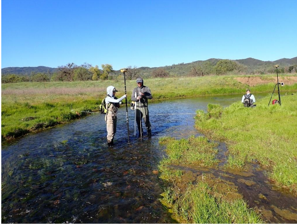
Figure D-1. CDFW field staff measuring depth, velocity, and GPS coordinates on Adobe Creek near Adobe Reservoir, April 2024.
