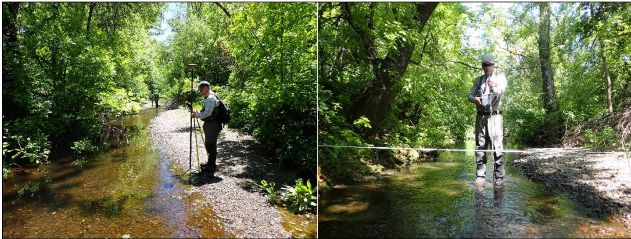
Figure C-4. CDFW field staff measuring water surface elevation and discharge on Manning Creek near Soda Bay Road, April 2024.
