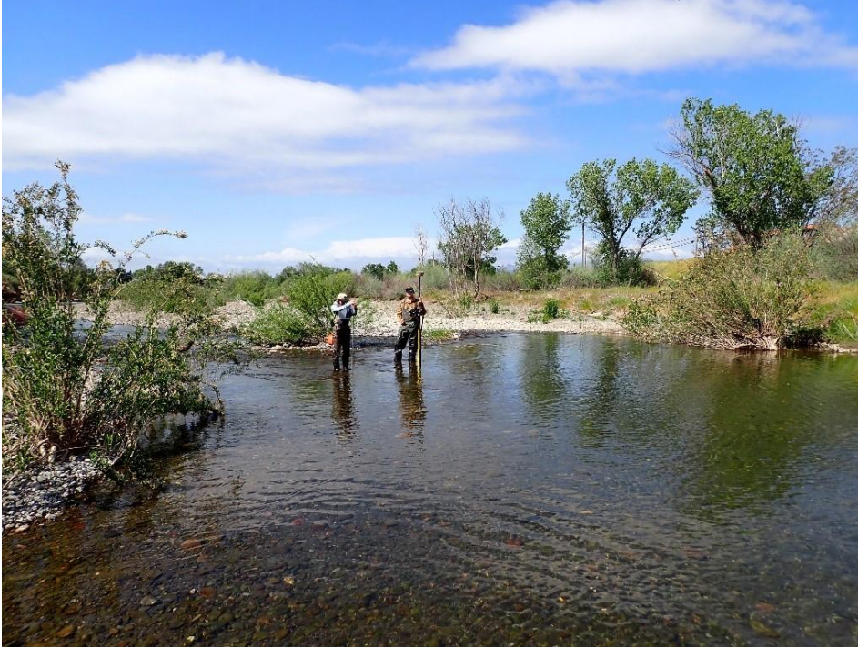
Figure D-3. CDFW field staff measuring depth, velocity, and GPS coordinates on Kelsey Creek near Finley East Road, April 2024.
