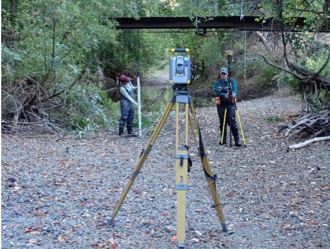
Figure B-3. Total station survey setup near a lidar void under a bridge on Scotts Creek, October 2024. The total station is in the foreground, with an RTK-GPS rover (right) and stadia rod with total station prism reflector (left) in the background.
