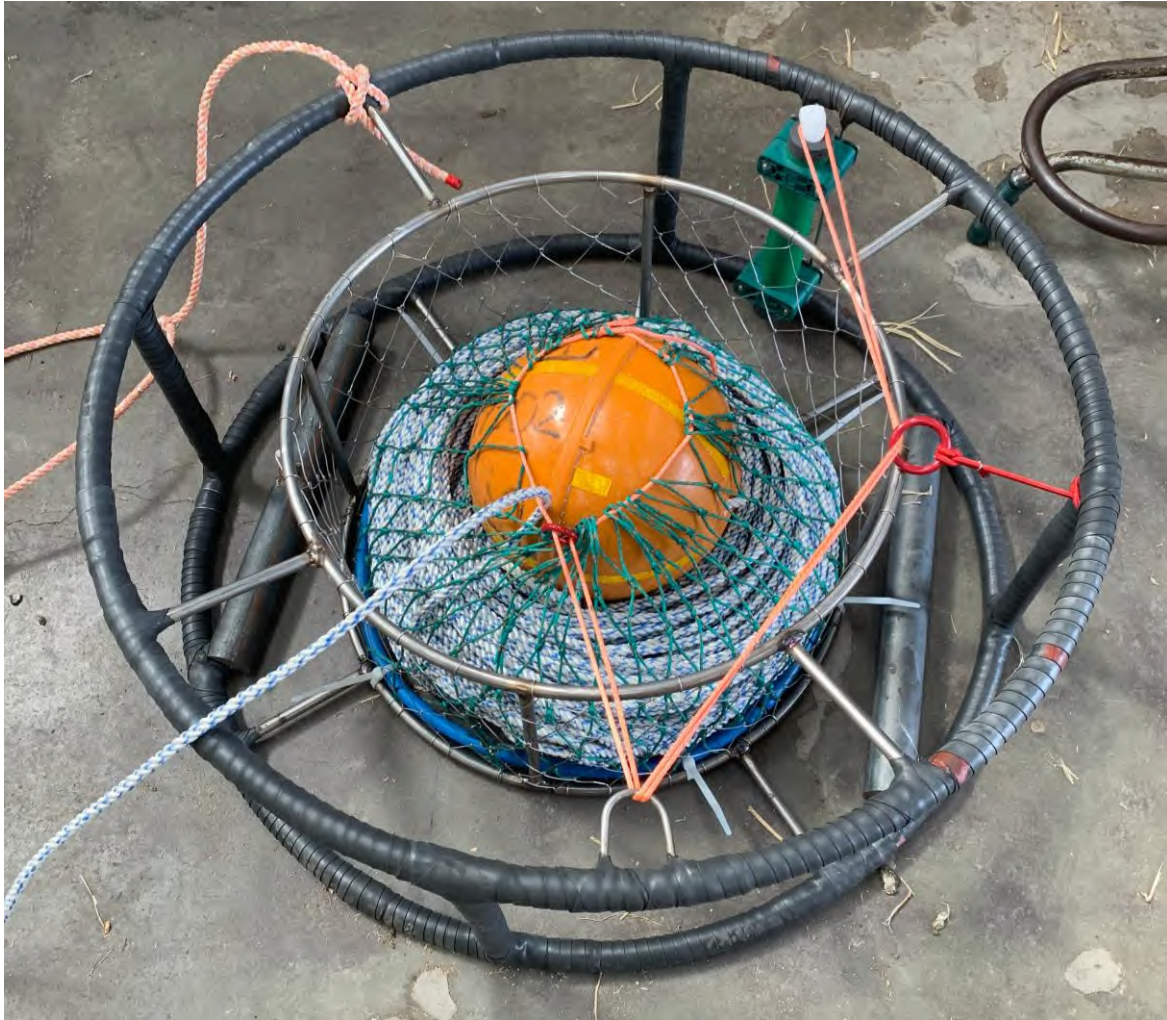
Figure 6. The Guardian Inshore Sled with Dungeness crab trap configuration.
