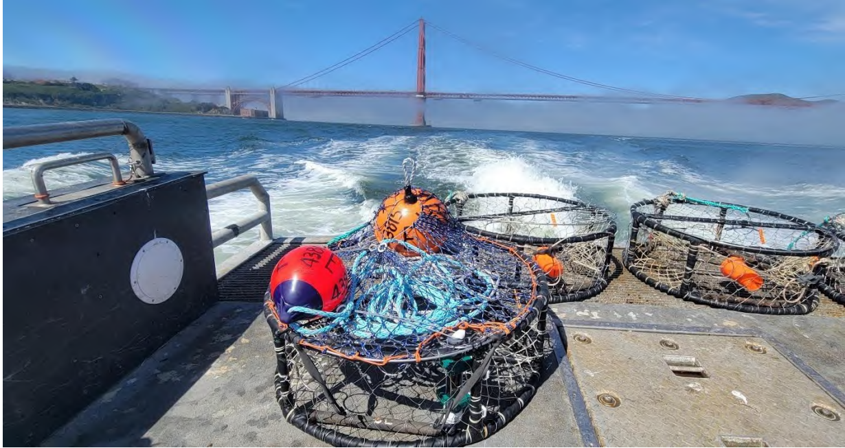
Figure 7. Trap-top retrofit Guardian line handling system.
