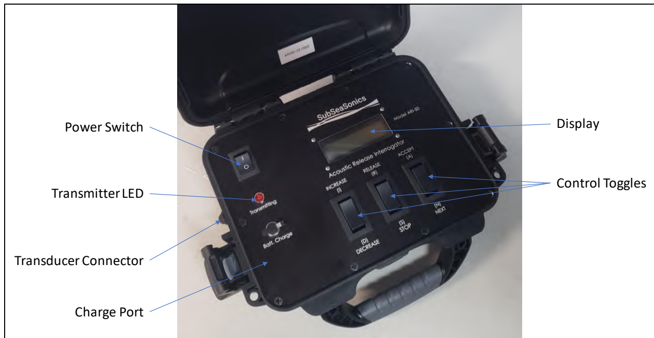
Figure 4. The ARI-U universal deck unit.
