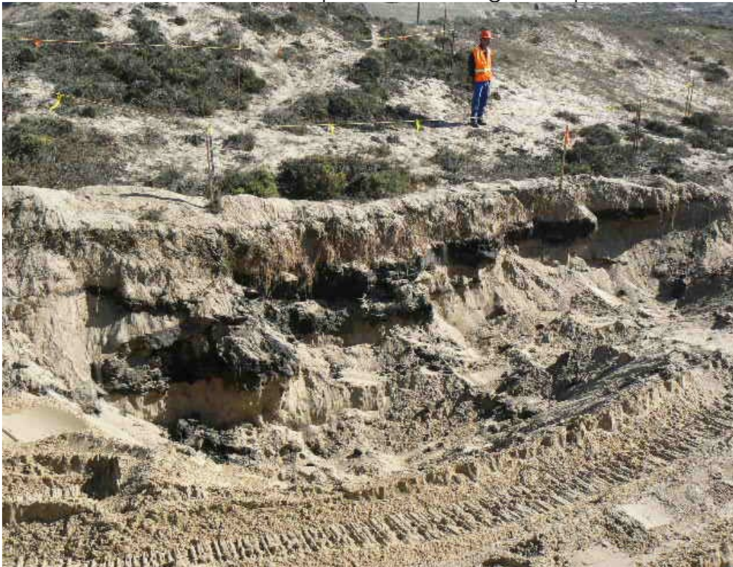
Photo 6. 2006 old, buried sump material along the supratidal zone.
