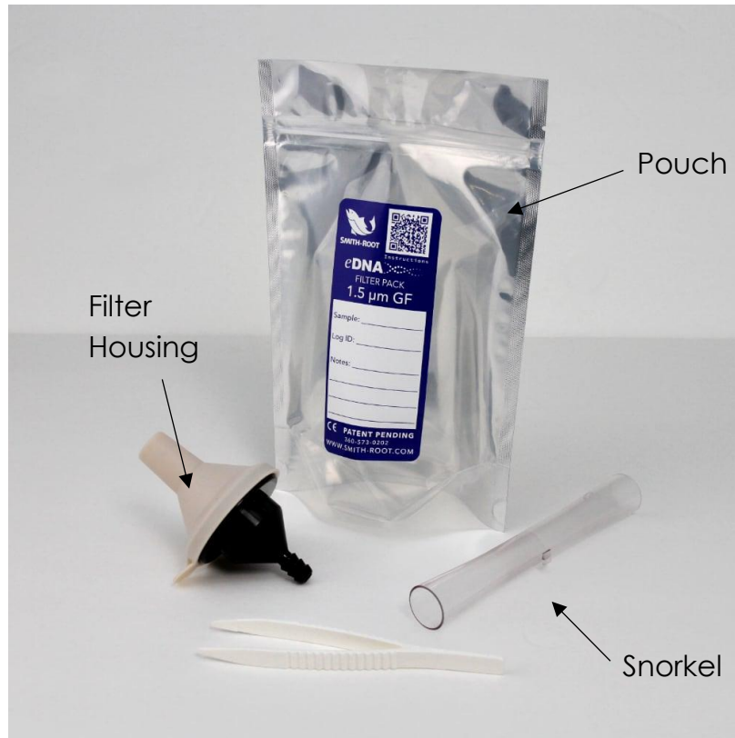
Figure 2. A Smith-Root filter pouch containing the filter housing and the snorkel.
